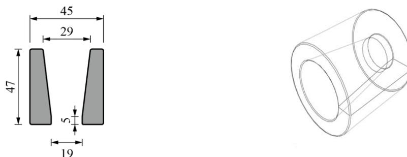
Fig. 1 Initial model of the tubular body (unit: mm)
