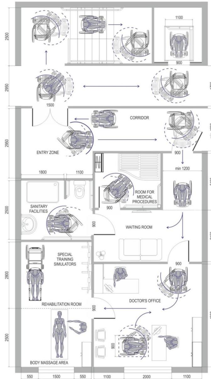
Fig. 11 Graphical analysis of optimal model of transportation in medical center
