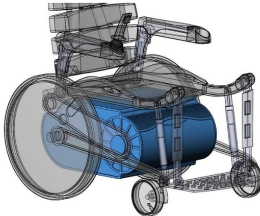
Fig. 8 The energy block of the wheelchair
