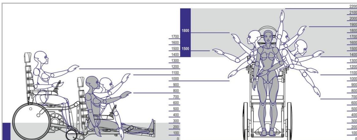
Fig. 6 Ergonomic scheme of the wheelchair
