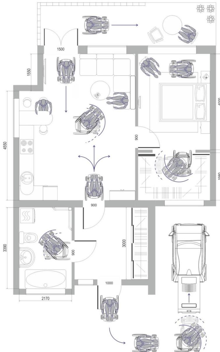
Fig. 10 Graphical analysis of optimal model of transportation in the house
