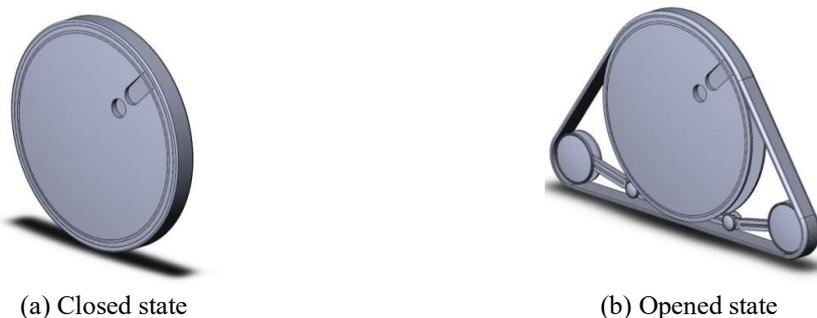
Fig. 2 Transformation of “Galileo Wheel” with two wheelpairs
