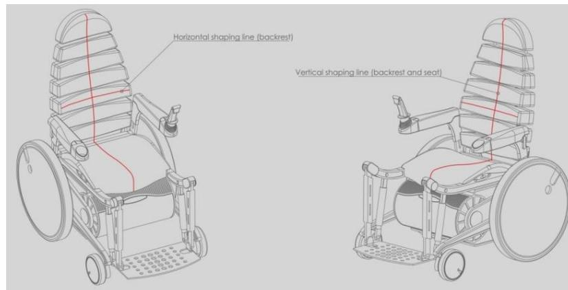
Fig. 5 Shaping lines of the backrest and seat with parameters provided by B. Akerblom
