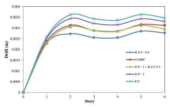
Fig. 15 Drift results of 6 story frame (R.Z.F. = 0.5, D.P. = 2.0)
