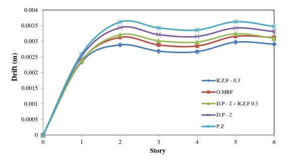
Fig. 14 Drift results of 6 story frame (R.Z.F. = 0.3, D.P. = 2.0)
