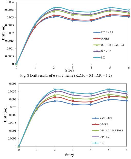
Fig. 9 Drift results of 6 story frame (R.Z.F. = 0.3, D.P. = 1.2)
