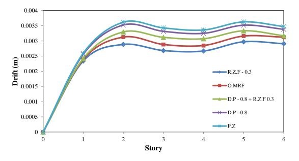
Fig. 4 Drift results of 6 story frame (R.Z.F. = 0.3, D.P. = 0.8)
