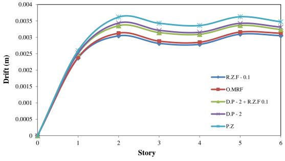
Fig. 13 Drift results of 6 story frame (R.Z.F. = 0.1, D.P. = 2.0)
