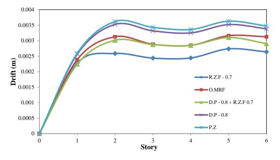
Fig. 6 Drift results of 6 story frame (R.Z.F. = 0.7, D.P. = 0.8)
