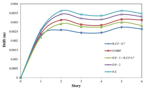
Fig. 16 Drift results of 6 story frame (R.Z.F. = 0.7, D.P. = 2.0)
