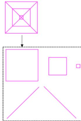
Fig. 3 Example of decomposed symbol (supply diffuser)
