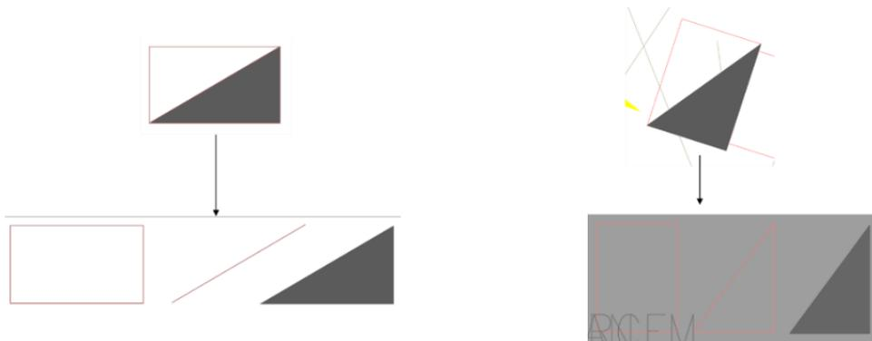
(a) Return air duct symbol from the symbol description document (b) Return air duct symbol from the actual 2D drawing
