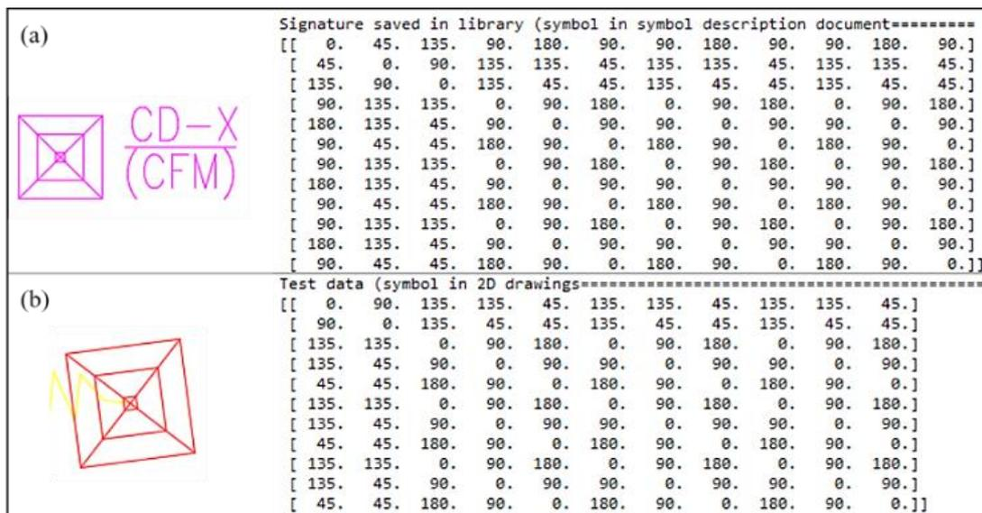
Fig. 5 Vectorial signature of the diffuser symbol (a) signature of the symbol in the symbol description document, (b) signature of the symbol in the 2D drawing (from Cho *et al.* 2018b)
