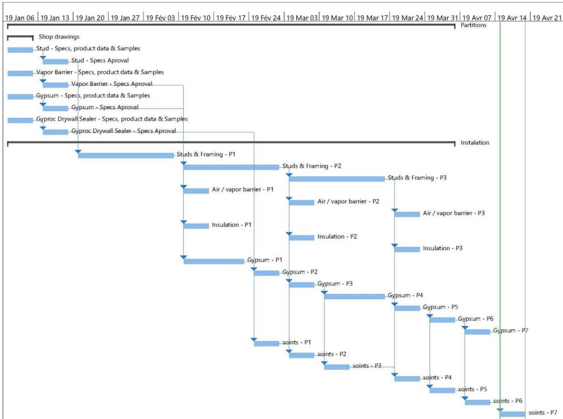
Fig. 5 Gantt-Precedence diagram for wall-partition planning
