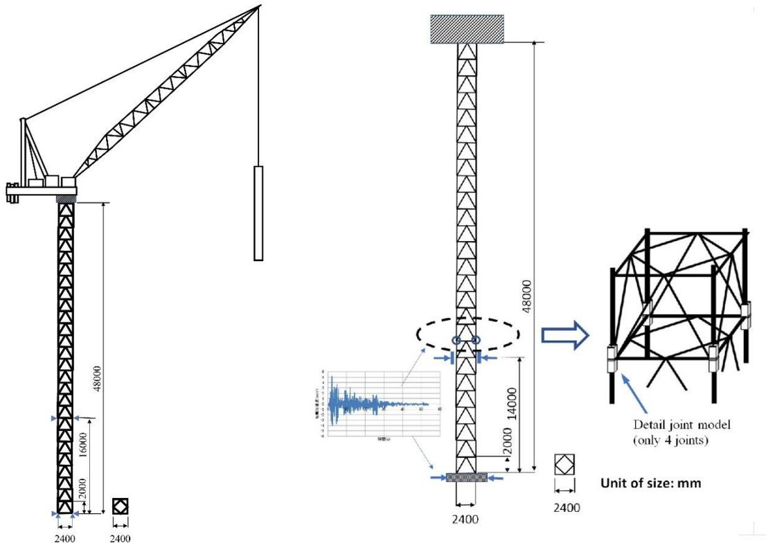
Fig. 2 Image of the analysis model for the FEM dynamic elastoplastic analysis of the tower crane
