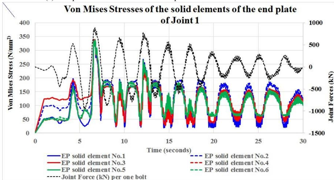
(b) Time-related responses of von Mises stress of the solid elements of an end-plate
