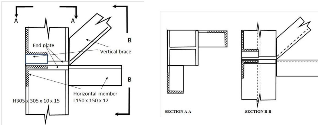
Fig. 6 Detail of a site-joint of the actual tower-crane mast
