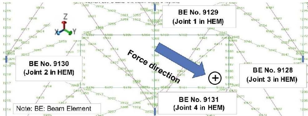
Fig. 14 Beam-elements of the joints and their numbers in the BEM
