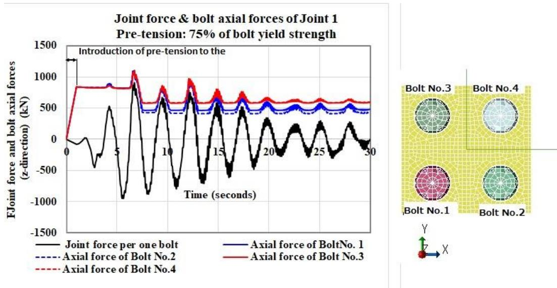
Fig. 18 Responses of bolt axial force and joint force on Joint 1
