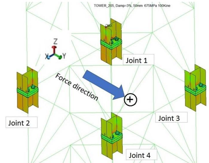
Fig. 15 Detailed model joints and their numbers in the HEM
