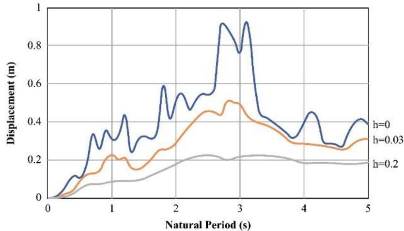
Fig. 10 Displacement spectra of El Centro N-S waves
