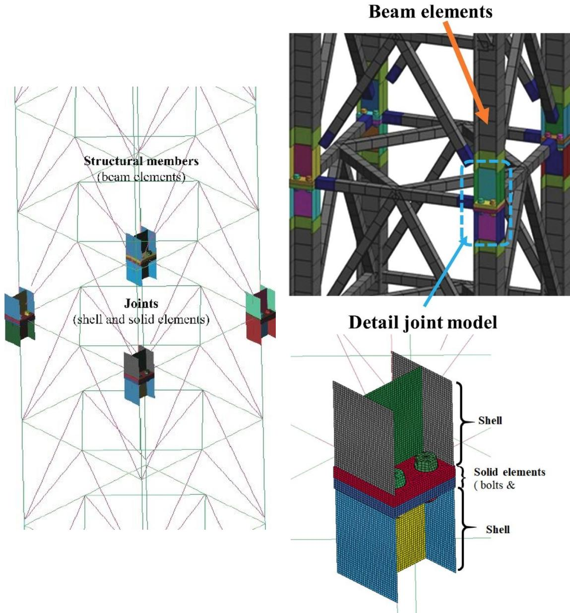
Fig. 3 Modeling of the tower-crane mast (three-dimensional truss and end-plate type bolted site-joint)
