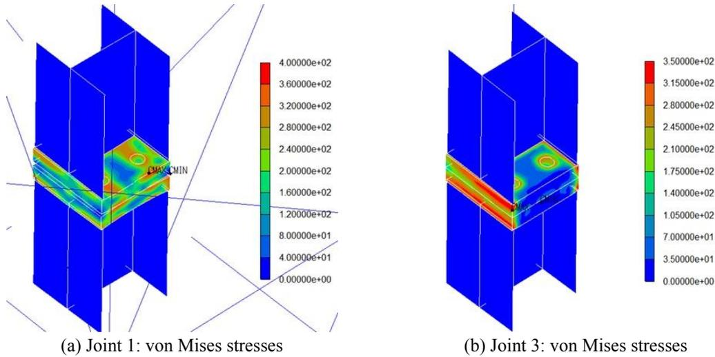
Fig. 20 Contour plot of the von Mises stress for Joints 1 and 3 at 6.72 s
