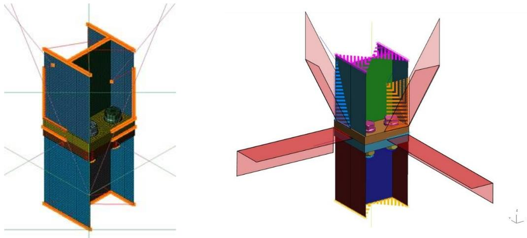
Fig. 7 Modeled connections between the end-plate-type bolt joint, horizontal members, and vertical bracings
