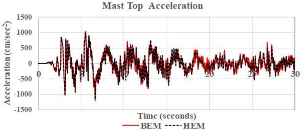
Fig. 13 Acceleration history of the tower-crane top (BEM and HEM)
