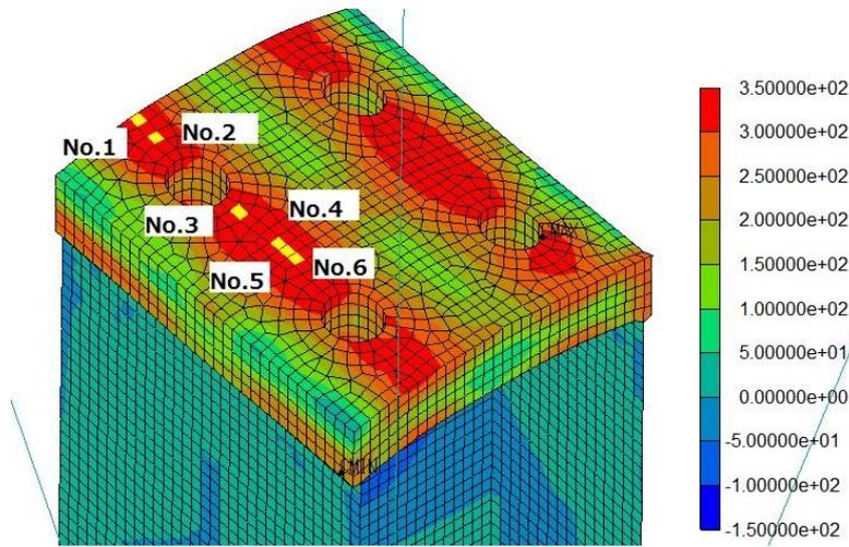
(a) End-plate von Mises stress contour plots and the solid-element numbers
