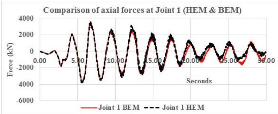
Fig. 16 Comparison of axial forces between HEM and BEM at Joint 1
