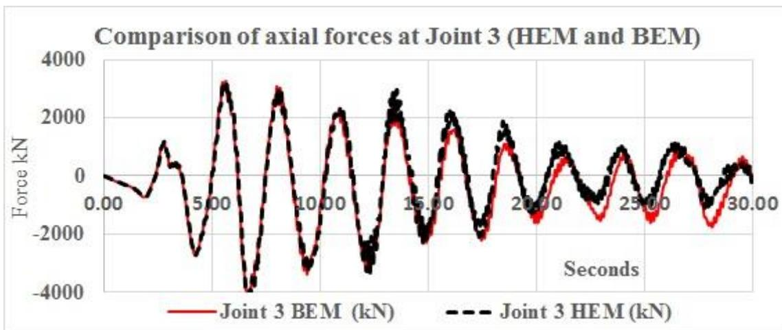
Fig. 17 Comparison of axial forces between HEM and BEM at Joint 3
