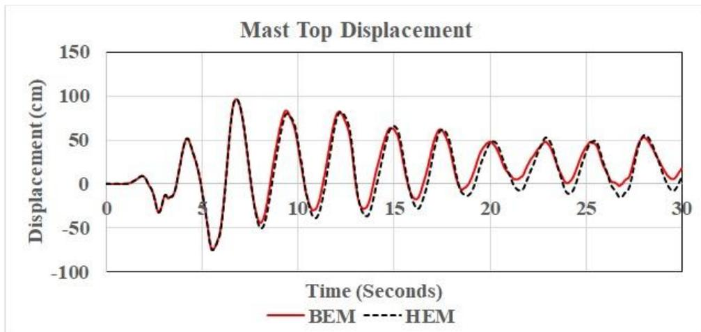
Fig. 12 Displacement history of the tower-crane top (BEM and HEM)
