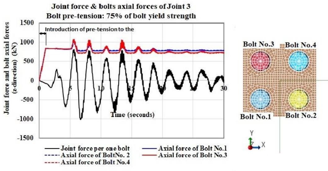
Fig. 19 Response bolt axial force and joint force on Joint 3
