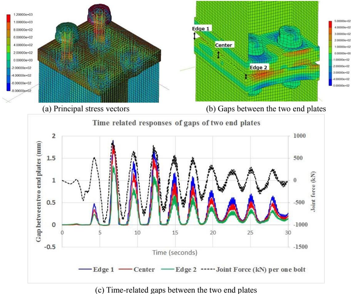
Fig. 23 Gap between the two end plates and the principal stress vectors
