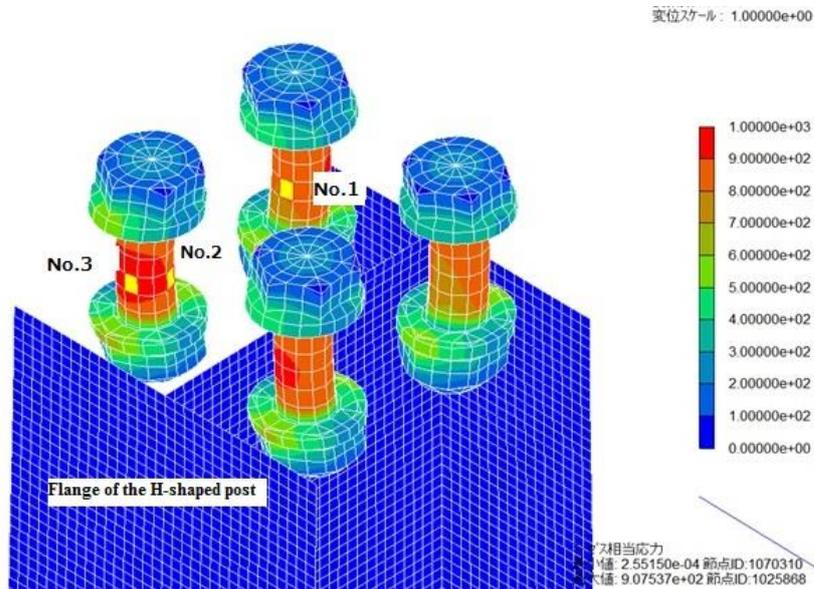
(a) Contour plots and solid-element numbers of the bolts in (b)
