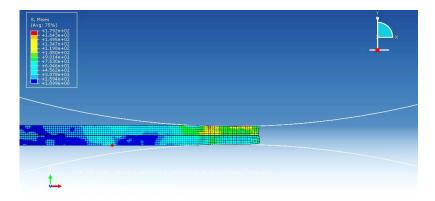
Fig. 4 Asymmetric rolling process of bimetal Al/Cu laminates
