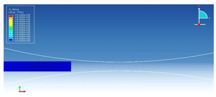
Fig. 3 Geometry and FE meshing of the asymmetric roll bonding process
