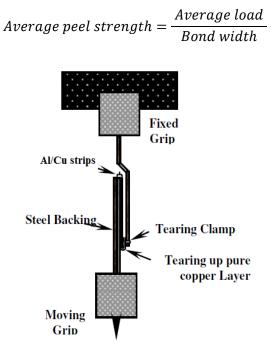
Fig. 2 Schematic illustration of the peeling test fixture
