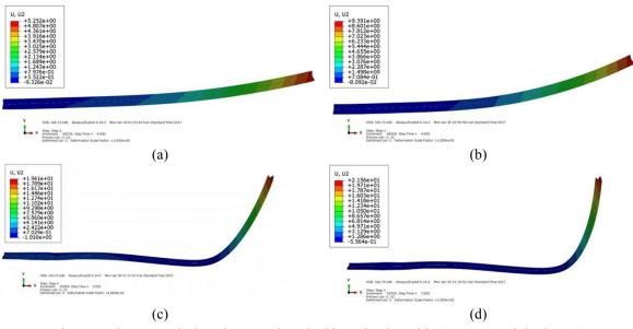
Fig. 5 Maximum vertical strain exerted on the bimetal strips with. (a, c) 1:1 and (b, d) 1:1.2
