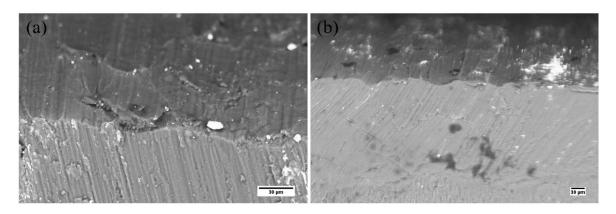
Fig. 7 SEM microstructure of as-rolled clad sheet with different mismatch speed ratios (a) 1:1 and (b) 1:1.2
