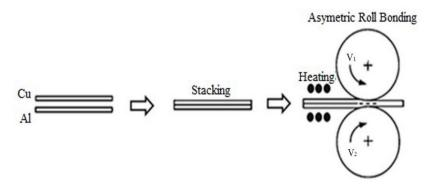
Fig. 1 Schematic diagram of asymmetrical RB process
