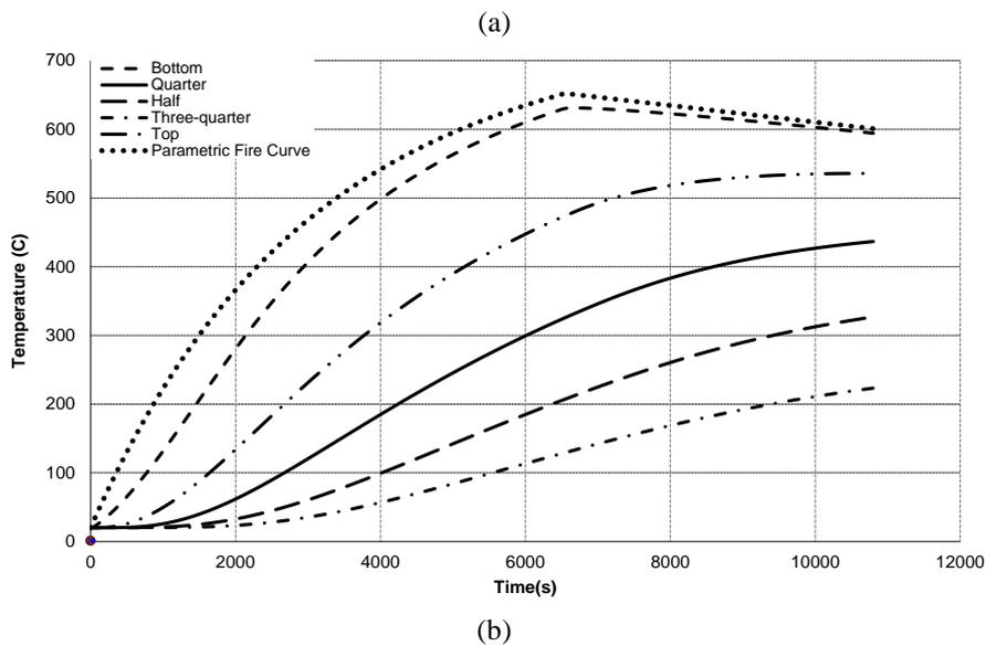
Fig. 4 Heat transferring result of slab and parametric fire temperature curve
