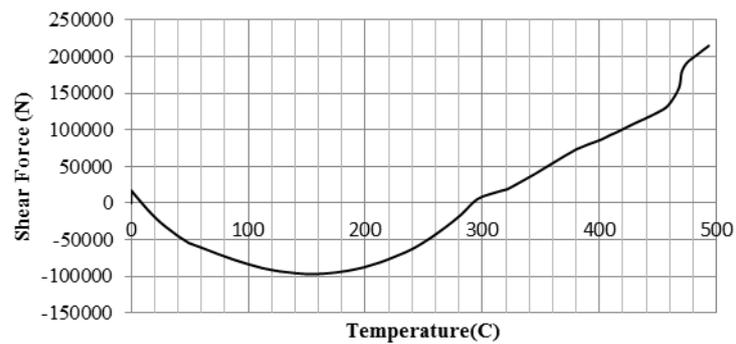
Fig.13 Shear Force of Column A1 at floor 10
