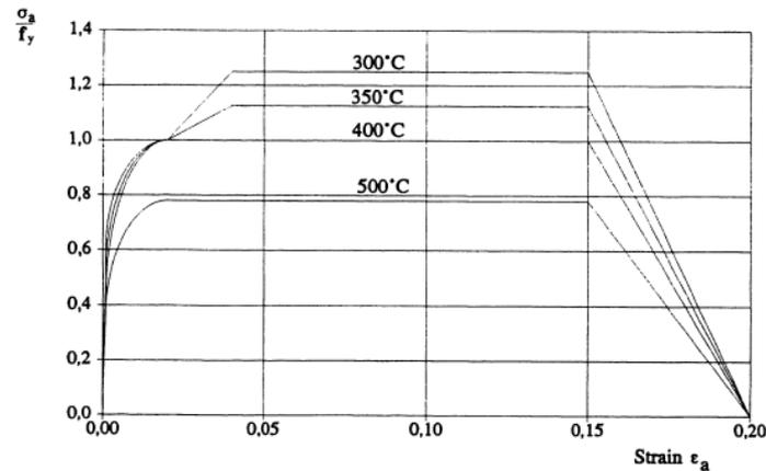
Fig. 5 Stress-strain relationship of structural steel at elevated temperature, allowing for strain hardening ENV 1993-1-2 (1995)
