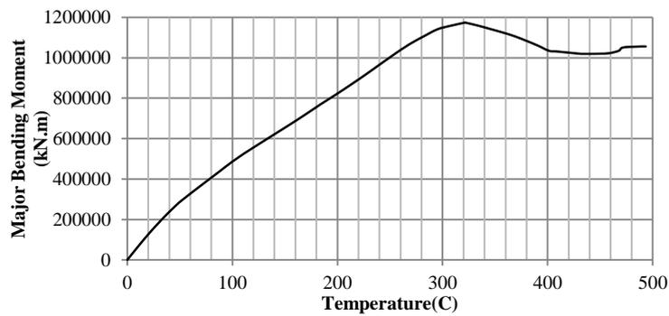
Fig. 12 Major Bending moment of Column A1 at floor 10
