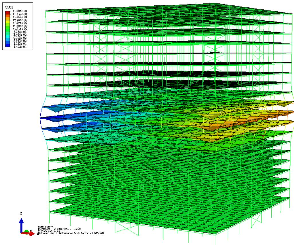
Fig. 10 Horizontal deflection of the model (deformation is amplified)
