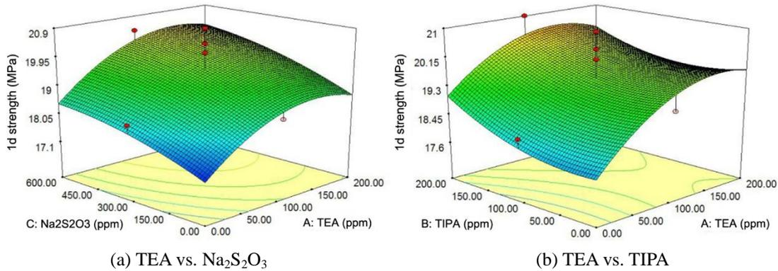
Fig. 4 Impacts of chemicals on 1d strength of cement
