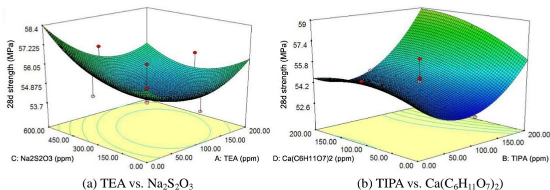
Fig. 6 Impacts of chemicals on 3d strength of cement
