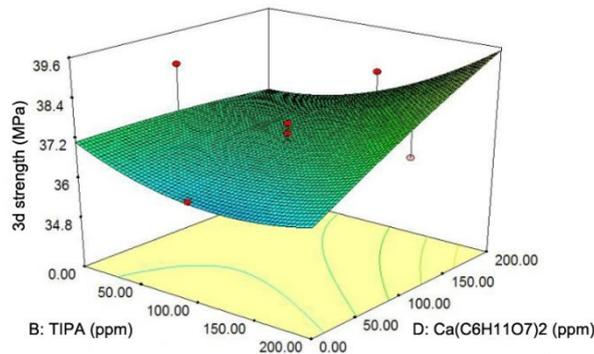
Fig. 5 Impacts of chemicals on 3d strength of cement (TIPA vs.  $\text{Ca}(\text{C}_6\text{H}_{11}\text{O}_7)_2$ )
