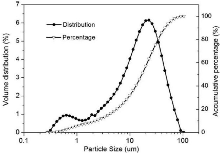
Fig. 2 Particle size distribution of 42.5R cement
