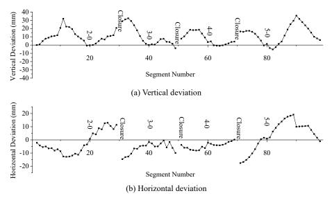
Fig. 18 Deviations in the segment alignment in erection phase
