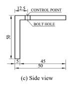
Fig. 11 Stainless steel marker (units: mm)
