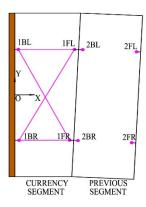
Fig. 10 Geometry control measurements in the four-point method
