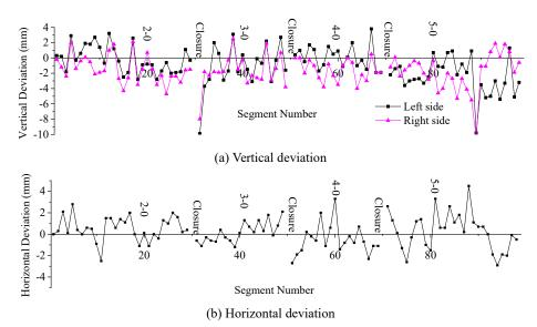
Fig. 17 Deviations in the segment alignment in the precast phase
