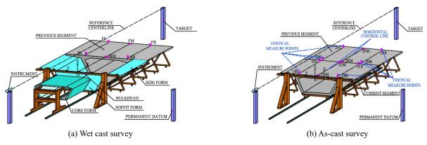
Fig. 3 Geometry survey system in the six-point method
