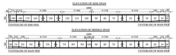
Fig. 13 Segment layout of the Leqing Bay Bridge (units: cm): (a) elevation of the side span; and (b) elevation of the middle span
