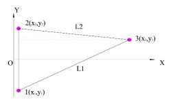
Fig. 9 Coordinate calculation of the unknown point
