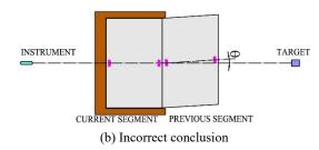
Fig. 6 Segment positions when unexpected offset occurs
