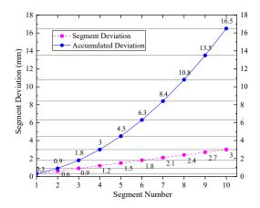
Fig. 8 Horizontal accumulated deviation as a result of one unexpected horizontal offset in the target
