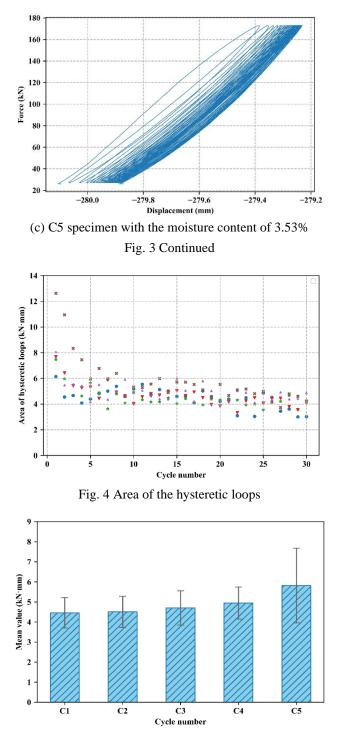
Fig. 5 Mean value and standard deviation of the areas of the hysteretic loops
