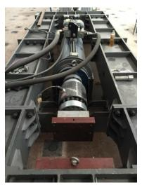
(a) Electric-hydraulic servo multi-function testing machine Fig. 1 Test setup
