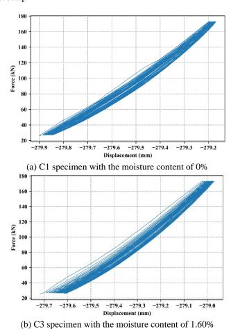
Fig. 3 Experimental hysteretic loops with different moisture contents
