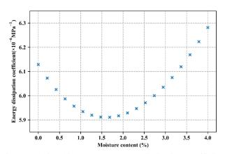
Fig. 8 Relationship between energy dissipation coefficient and moisture content
