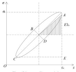
Fig. 6 Diagram of hysteresis loop
