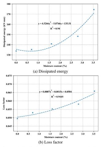
Fig. 7 Relationship between dissipated energy dissipation property and moisture content
