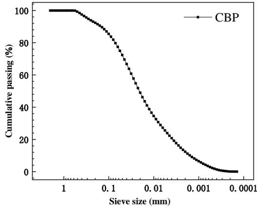
Fig. 1 Particle size distribution curve of clay brick powder
