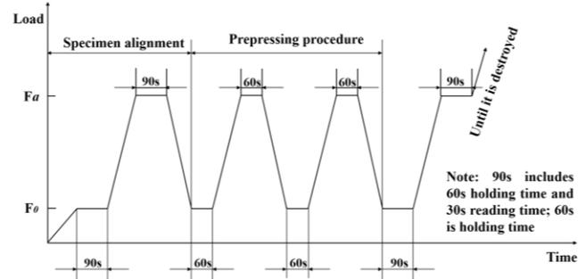
Fig. 2 Loading system for elastic modulus test
