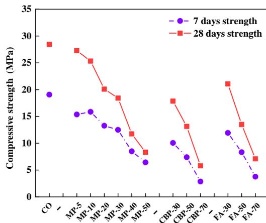
Fig. 4 Effects of different substitution groups on compressive strength
