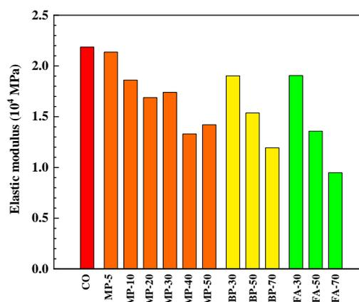
Fig. 5 Effects of different substitution groups on elastic modulus
