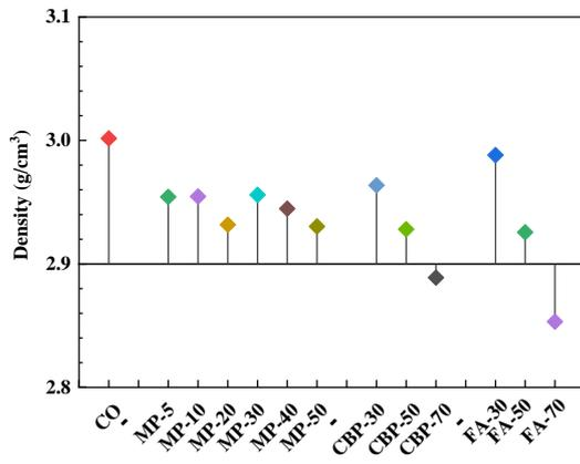
Fig. 3 Effects of different substitution groups on density
