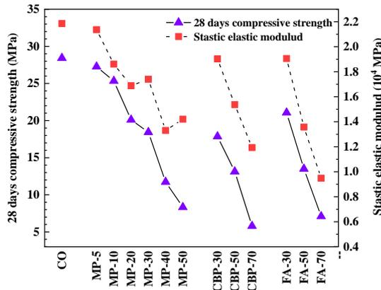
Fig. 6 Comparison of compressive strength and elastic modulus values of different substitution groups
