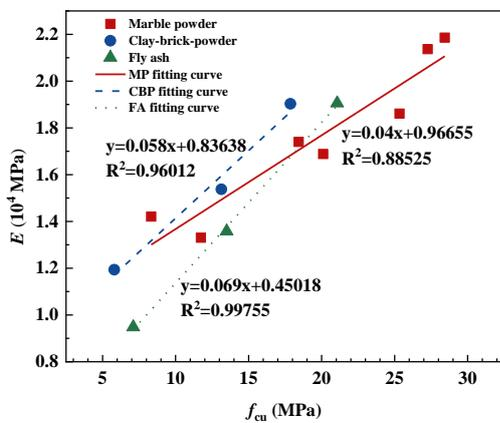
Fig. 7 Relationship between compressive strength and elastic modulus
