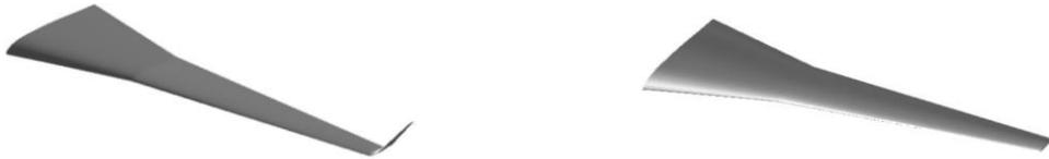
Fig. 5 Geometry of simple and blended wing of Boeing 737-800 aircraft
