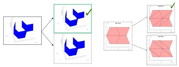
(a) Core hexagonal cell mesh triangularization
