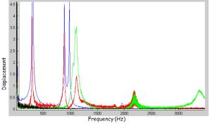
(a) Honeycomb sandwich panel SS (b) FTF frequency responses (colors indicate configuration
