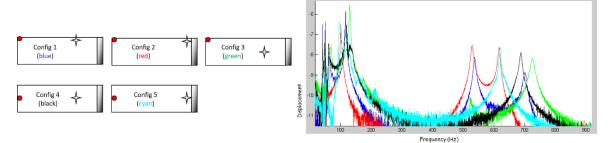
(a) Excitations (red discs) and measurements (b) First few modes Fourier Transfer Functions (FTF) (stars) normal to the clamped (shaded area) panel
