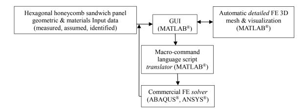
Fig. 6 Flowchart of the proposed practical, simplified and detailed FE 3D modelling approach of the actual GFRP-Epoxy woven composite-aluminum alloy hexagonal honeycomb sandwich panel
