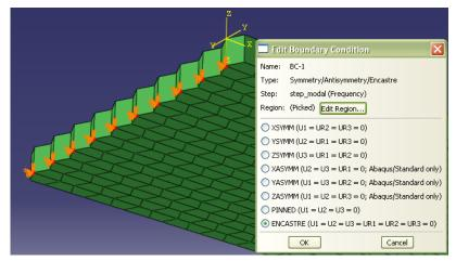
Fig. 9 Modelling of the adhesive glue beads for the actual SS configuration of Fig. 5a
