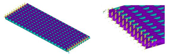
(a) SS BCs modelling (b) Cantilever BCs modelling Fig. 11 Implementation for ANSYS<sup>®</sup> of the SS and cantilever BCs using the detailed FE 3D approach
