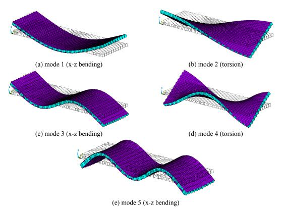
Fig. 12 Hexagonal honeycomb sandwich panel simulated first 5 modes under free BCs using ANSYS1
