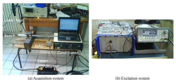
Fig. 2 Experimental setup for the free-vibration of the honeycomb sandwich panel (here cantilevered)
