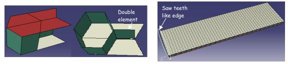
(a) Hexagonal honeycomb core mesh basic cell(b) Detailed FE 3D mesh of the sandwich panelFig. 7 Hexagonal honeycomb sandwich panel detailed 3D mesh by the developed MATLAB<sup>®</sup> mesh tool
