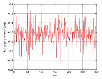
Fig. 7 Rhe variation of the roll angle error mean in the Monte-Carlo runs
