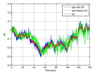
Fig. 3 The third component of the estimated and true quaternion
