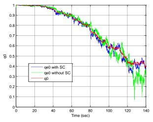
Fig. 4 The scalar component of the estimated and true quaternion
