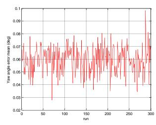
Fig. 5 The variation of the yaw angle error mean in the Monte-Carlo runs
