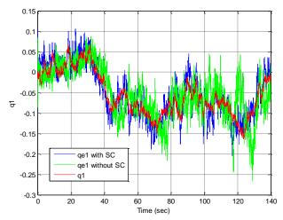
Fig. 1 The first component of the estimated and true quaternion
