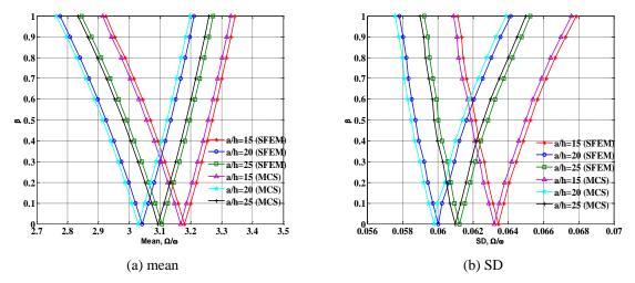
Fig. 7 Effect of theslenderness ratios on the dynamic instability region with random material properties  $\{b_i(i=1,...,10)=0.1\}$  of piezoelectric FGM beams
