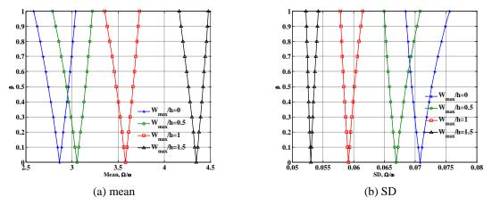
Fig. 10 Effect of the amplitude ratios ( $W_{\text{max/h}} = 0$ , 0.5, 1, 1.5) on the dynamic instability region of piezoelectric FGM beams with random material properties.
