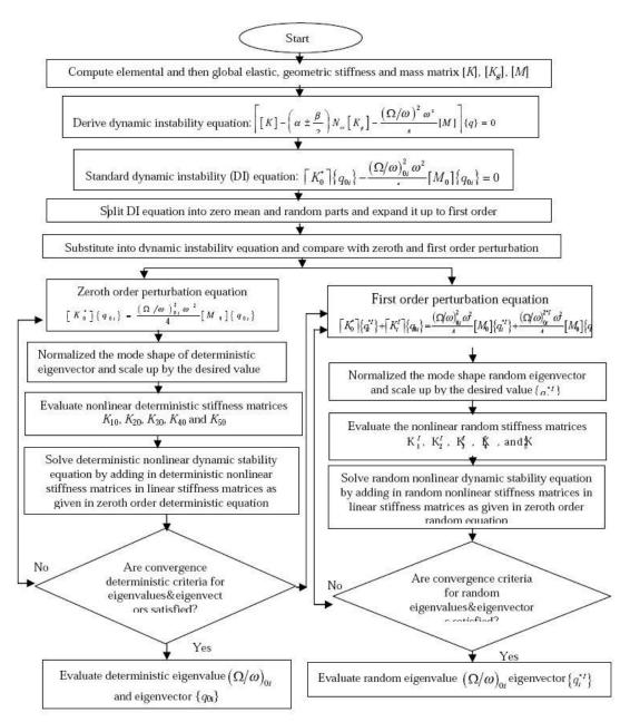
Fig. 2 Flow chart of solution procedure of stochastic dynamic stability analysis
