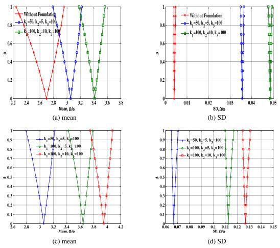
Fig. 11 Effect of thefoundation parameters on the dynamic instability of piezoelectric FGM beam
