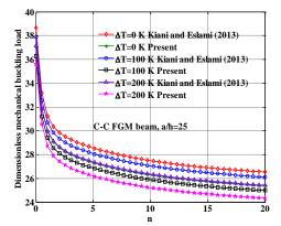
Fig. 5Validation study for variation of volume fraction exponents with temperature change on the mechanical buckling of FGM beam
