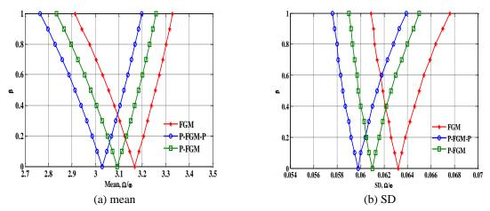
Fig. 14 Effect of theposition of piezoelectric layer on the dynamic instability of piezoelectric FGM beams
