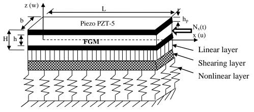
Fig. 1 Geometry of a piezoelectric FGM beam supported by elastic foundation
