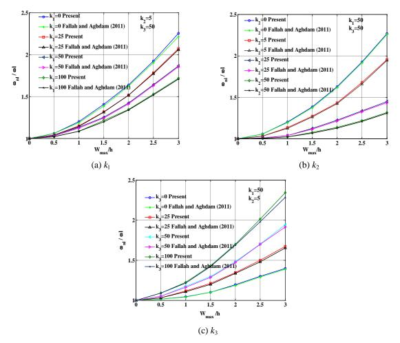
Fig. 4 Validation studyfor variation of amplitude ratios with foundation parameters  $k_1$ ,  $k_2$  and  $k_3$  on the frequency ratio of simply supported functionally graded beam
