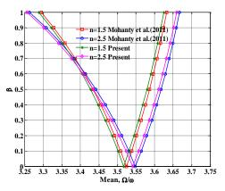
Fig. 6 Comparison of the primary instability regions versus dynamic in-plane load parameters,  $\beta$  for FGM beam
