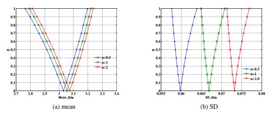
Fig. 12 Effect of thevolume fraction exponents on the dynamic instability region of piezoelectric FGM beam
