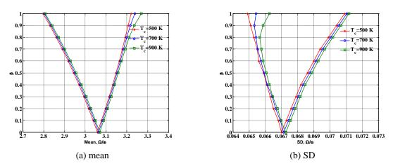
Fig. 13 Effect of thetemperature variation on top surface on the dynamic instability region of FGM beam
