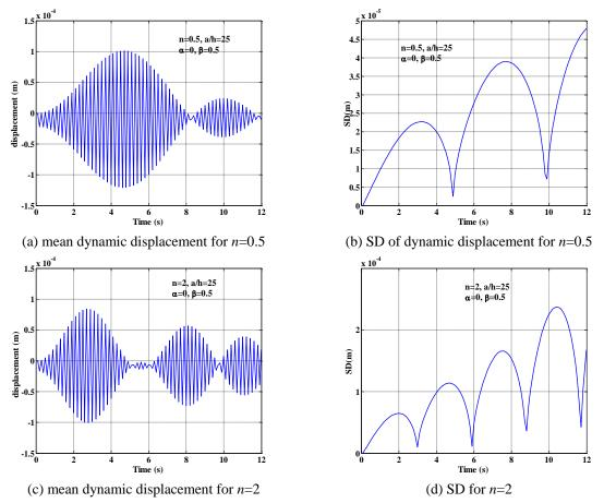
Fig. 17 Effect of volume fraction exponents on mean and SD of dynamic displacement
