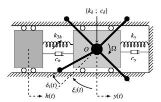
Fig. 3 Descriptive diagram of the used helicopter system coupled to an ungrounded NES. View from the top
