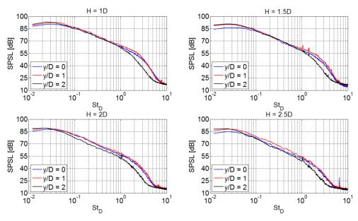
Fig. 9 Span-wise SPSL for x/D=25 at H/D=1, H/D=1.5, H/D=2 and H/D=2.5
