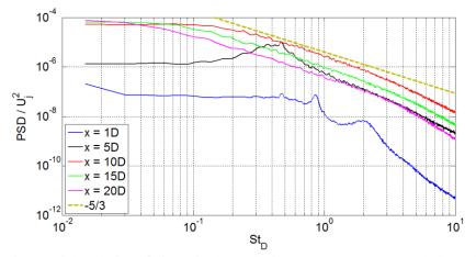
Fig. 6 Axial evolution of dimensionless velocity power spectra vs Strouhal number.
