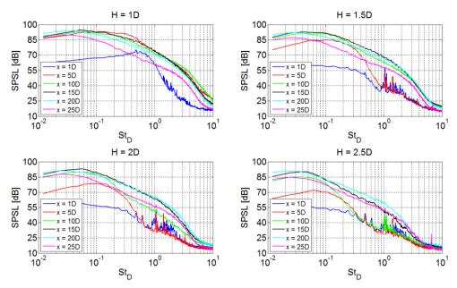
Fig. 7 Stream-wise SPSL evolution for y/D=0 at H/D=1, H/D=1.5, H/D=2 and H/D=2.5
