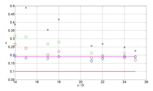
Fig. 14 Axial evolution of the Corcos' model stream-wise coefficient from x/D=14 to x/D=25 for flat plate distances: H/D=1; H/D=1.5; H/D=2; H/D=2. Solid line and dashed line refers respectively to the lower and upper limit values of the Corcos' model coefficient found in the literature
