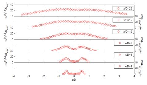
Fig. 5 Stream-wise turbulence intensity at different axial positions.
