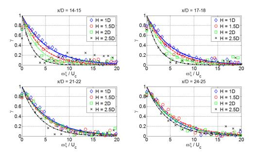
Fig. 12 Coherence functions and Corcos' model fits parametrized by the flat plate distance for different axial positions beyond the impact point
