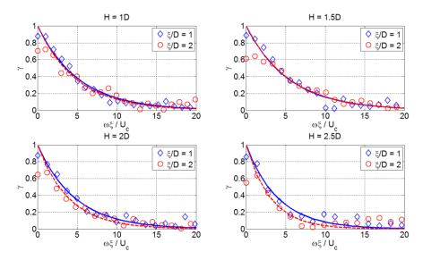
Fig. 16 Streamwise coherence and Corcos' model versus cross-spectral phase for 2 spacings  $\xi=1-2D$  at x/D=23 for all the flat plate radial distances
