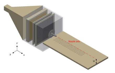
Fig. 2 Scheme of the pin-holes distribution on the flat plate and identification of the reference system. The parameter H represents the distance between the flat plate and the nozzle axis.
