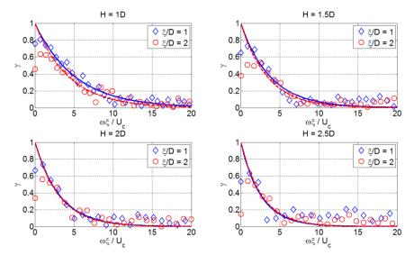
Fig. 15 Streamwise coherence and Corcos' model versus cross-spectral phase for 2 spacings  $\xi=1-2D$  at x/D=13 for all the flat plate radial distances
