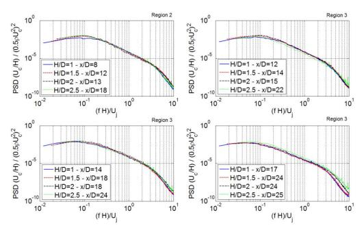
Fig. 11 Scaled spectra using outer variables as function of the flow evolution on the flat plate. For more details on the region definition, the reader is referred to Di Marco *et al.* (2015)
