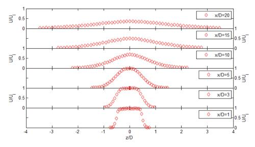
Fig. 4 Stream-wise mean velocity at different axial positions.
