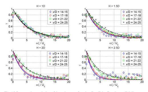
Fig. 13 Stream-wise evolution of the coherence function for all the flat plate radial distances
