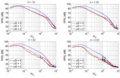
Fig. 8 Span-wise SPSL for x/D=15 at H/D=1, H/D=1.5, H/D=2 and H/D=2.5
