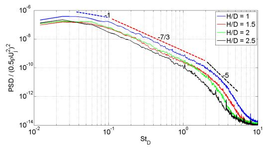
Fig. 10 Dimensionless PSDs at x/D=25 for the flat plate distances considered
