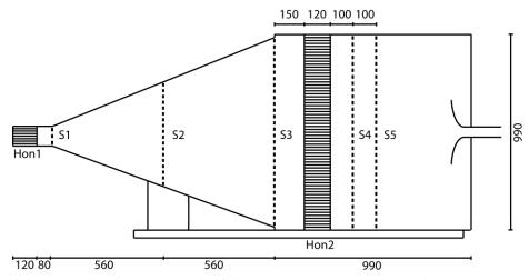
Fig. 1 Layout of the experimental free jet facility. The measures are in millimeters. The abbreviation Hon# indicates the honeycomb and S# the turbulence screen
