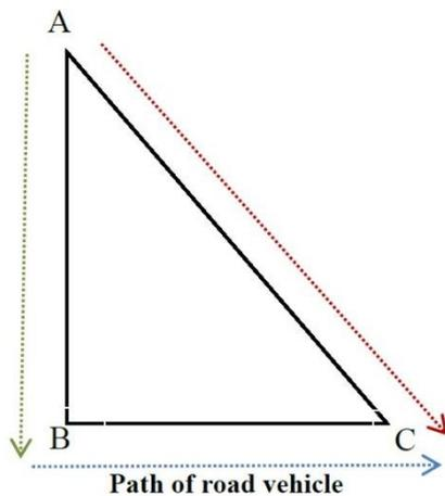
Fig. 3 Different travel distance between the drone and road vehicles with the same starting point and ending point
