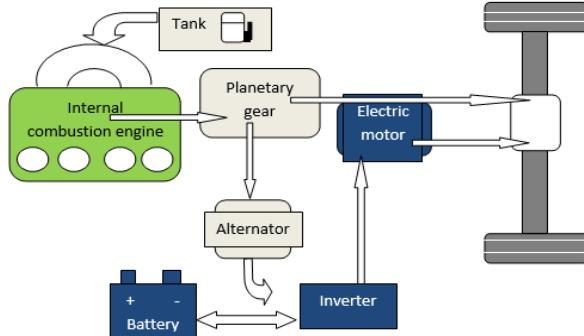
Fig. 4 Physical diagram of combined hybrid electric vehicle
