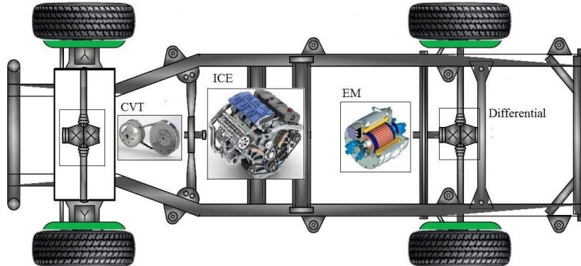
Fig. 1 The mechanical powertrain configuration
