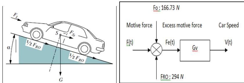
Fig. 8 Illustration of running resistances for a car moving uphill (Bosch 2007)
