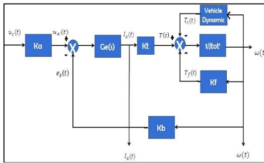
Fig. 5 The block diagram of a hybrid vehicle forward path
