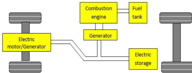
Fig. 2 Physical diagram of serial hybrid electric vehicle
