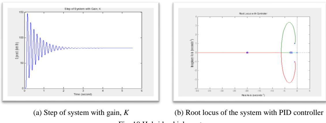
(a) Step of system with gain,  $K$  (b) Root locus of the system with PID controller
