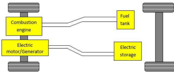
Fig. 3 Physical diagram of parallel hybrid electric vehicle
