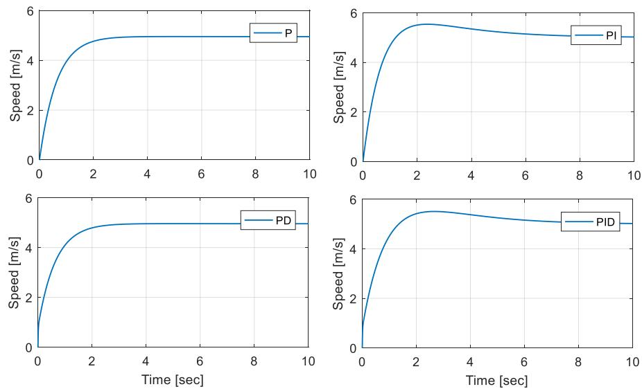
Fig. 11 Speed response for hybrid vehicle system through P, PI, PD, and PID
