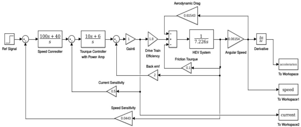
Fig. 6 Cascade control of the hybrid vehicle system
