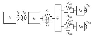
Fig. 2 Model of the driveline
