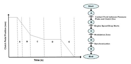
Fig. 5 Theoretical clutch pedal position during drive-off
