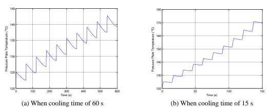
Fig. 16 Temperature of pressure plate during drive-off when the pedal travels with the same speed all the way in modulation zone
