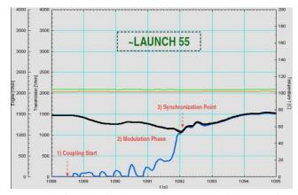
Fig. 21 Angular speeds of engine flywheel and transmission input shaft at 55th drive-off
