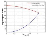
(a) The angular velocities of the engine flywheel and the transmission input shaft
