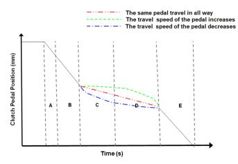
Fig. 6 Driver profiles for clutch pedal travel during slip time
