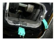
(a) The thermocouples on engine transmission assembly
