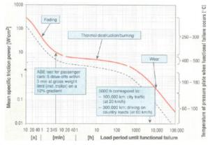
Fig. 15 The effect of mean friction power on the total clutch life (Coelho and Rabelo 2011)
