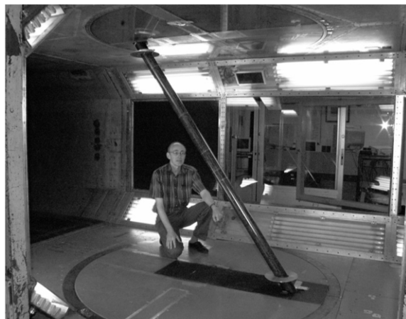
(b) Static model in the NRCC 2m x 3m wind tunnel
