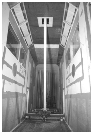
(a) Dynamic model in the NRCC 3m x 6m Propulsion wind tunnel
