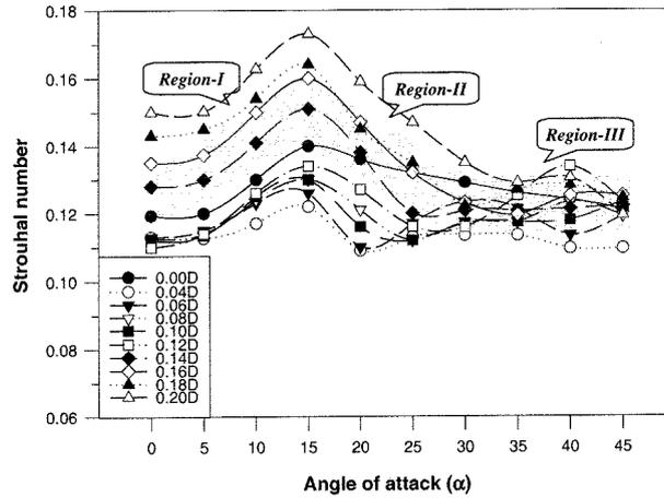
Fig. 6 Variation of the Strouhal numbers with angles of attack (B/D=1.0)
