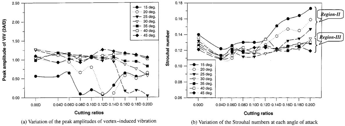
Fig. 10 The Strouhal number for B/D=1.0 with corner cuts
