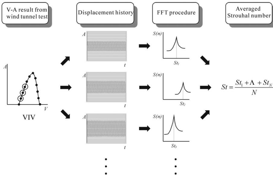
Fig. 3 Procedure of the proposed method to determine the Strouhal number
