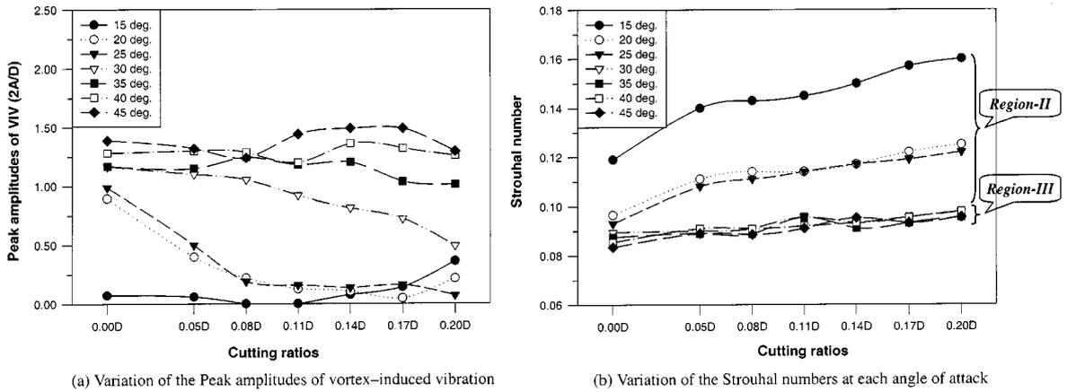
Fig. 12 The Strouhal number for B/D=1.5 with corner cuts
