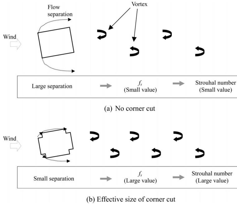
Fig. 11 A schematic diagram of flow separation and vortex-shedding
