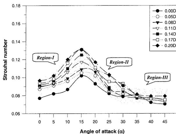
Fig. 8 Variation of the Strouhal numbers with angles of attack ( $B/D=2.0$ )
