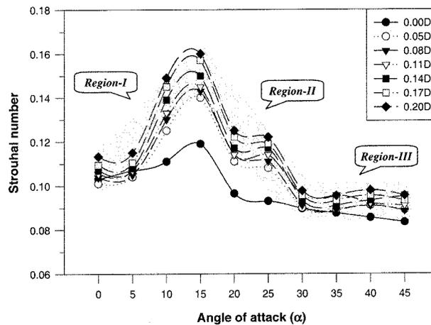
Fig. 7 Variation of the Strouhal numbers with angles of attack (B/D=1.5)
