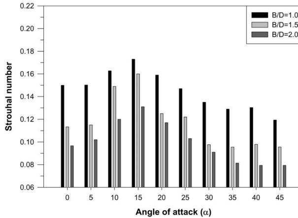
Fig. 9 Variation of the Strouhal numbers for corner cut size 0.20D
