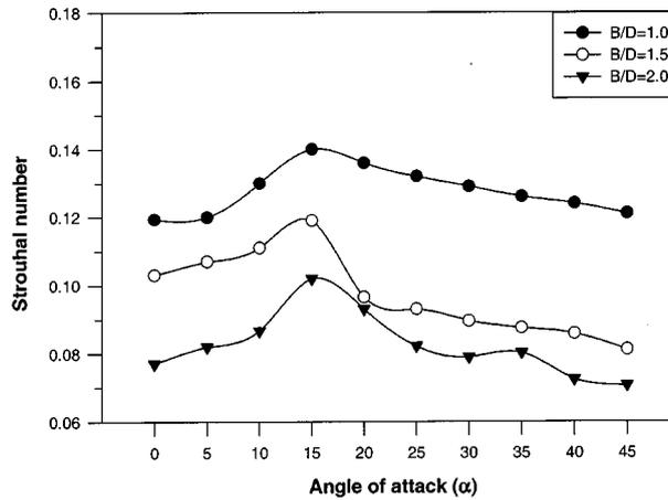
Fig. 4 Variation of the Strouhal numbers of rectangular cylinders without corner cut
