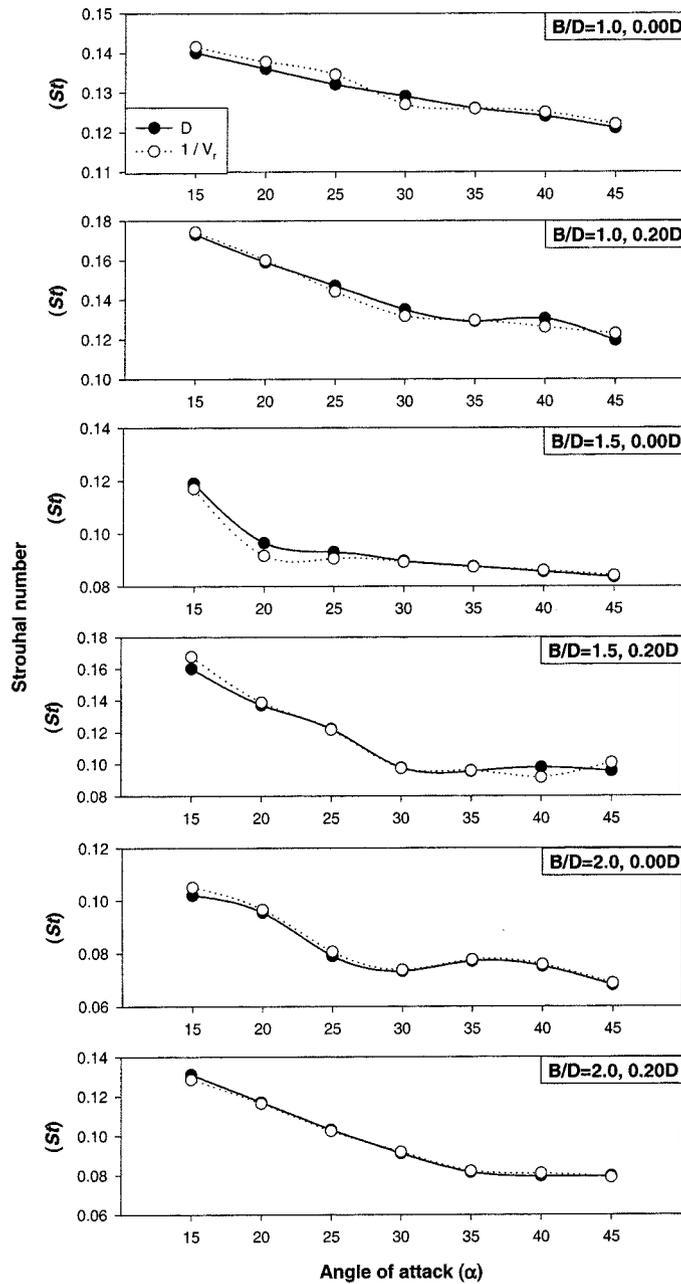
Fig. 5 Verification examples of the Strouhal number
