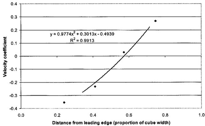
Fig. 7 Streamwise mean velocity close to the roof surface for  $0^\circ$  wind angle
