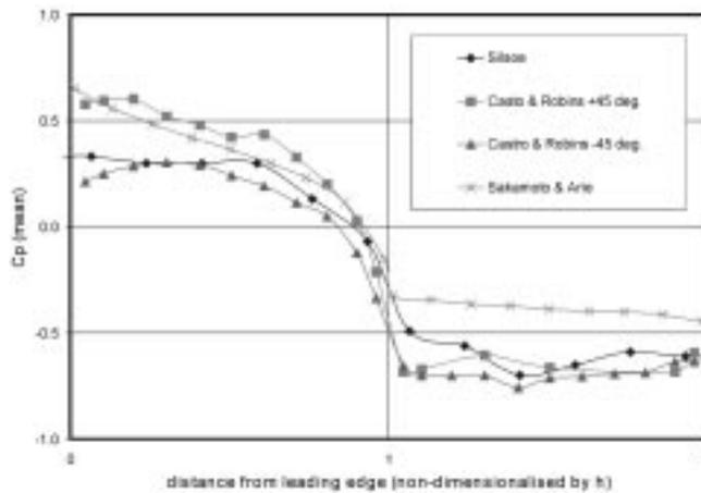
Fig. 12 Pressure distribution at mid height for  $45^\circ$  wind angel
