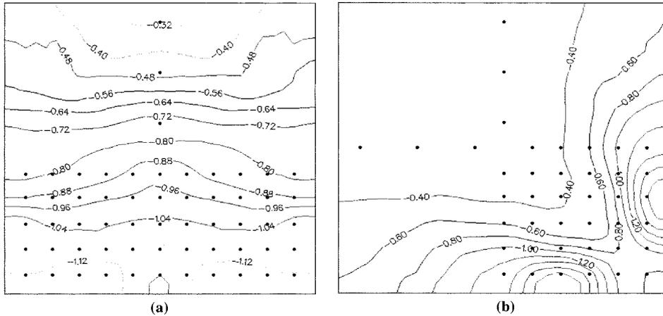
Fig. 5 (a) Pressure distribution on the roof for,  $0^\circ$  wind angle (b) Pressure distribution on the roof for,  $45^\circ$  wind angle
