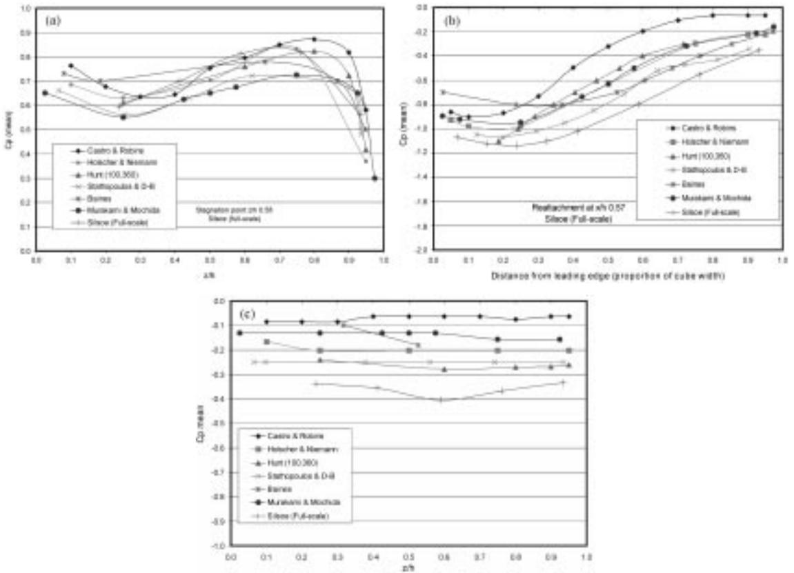
Fig. 9 (a) Pressure distribution on the windward face for  $0^\circ$  wind angle (b) Pressure distribution on the roof for  $0^\circ$  wind angle (c) Pressure distribution on the leeward wall for  $0^\circ$  wind angle
