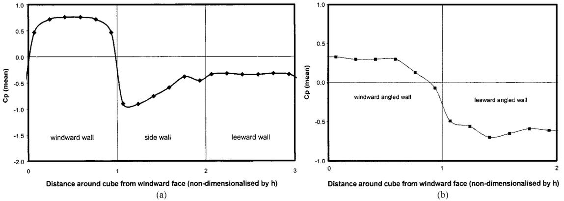
Fig. 4 (a) Pressure distribution at mid height for  $0^\circ$  wind angle (b) Pressure distribution at mid height for  $45^\circ$  wind angle
