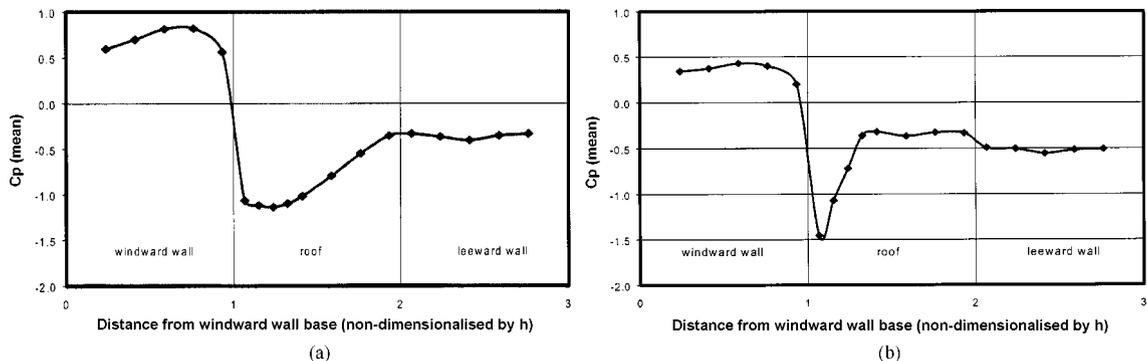
Fig. 3 (a) Pressure distribution around a vertical centreline for  $0^\circ$  wind angle (b) Pressure distribution around a vertical centreline for  $45^\circ$  wind angle
