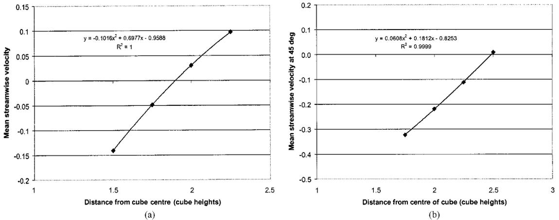
Fig. 8 (a) Streamwise mean velocity close to the ground behind the cube for  $0^\circ$  wind angle. (b) Streamwise mean velocity close to the ground behind the cube for  $45^\circ$  wind angle
