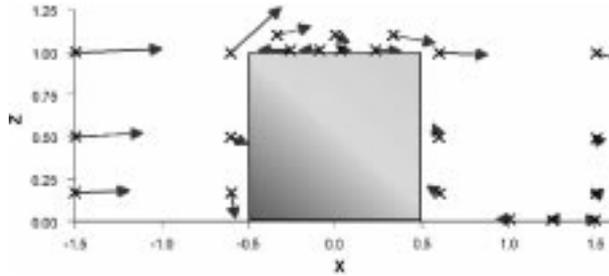
Fig. 6 Flow vectors measured on the cube centre plane  $y = 0$  (co-ordinates non-dimensionalised by  $h$ )
