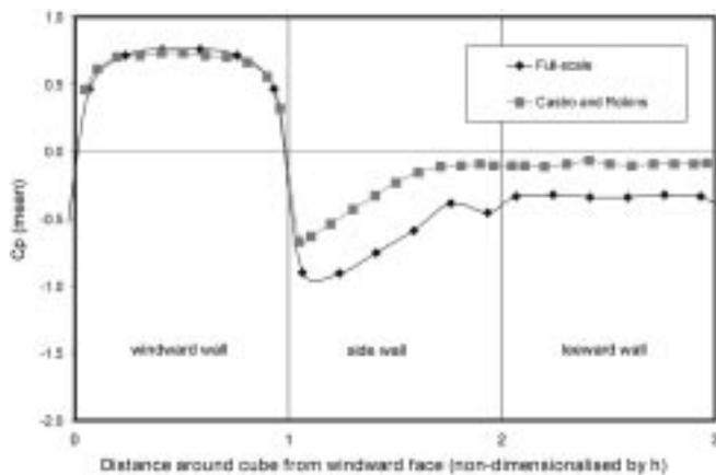
Fig. 10 Pressure distribution at mid height for  $0^\circ$  wind angle
