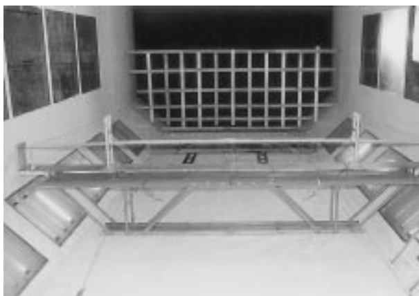
Fig. 8 Photo of the full bridge aeroelastic model in wind tunnel
