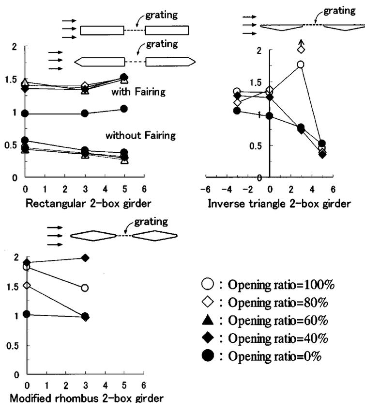
Fig. 12 Influence of angle of attack and grating opening ratio to flutter onset velocity. (horizontal axes: angle of attack (deg.), vertical axes: flutter onset velocity / that of thin plate case)
