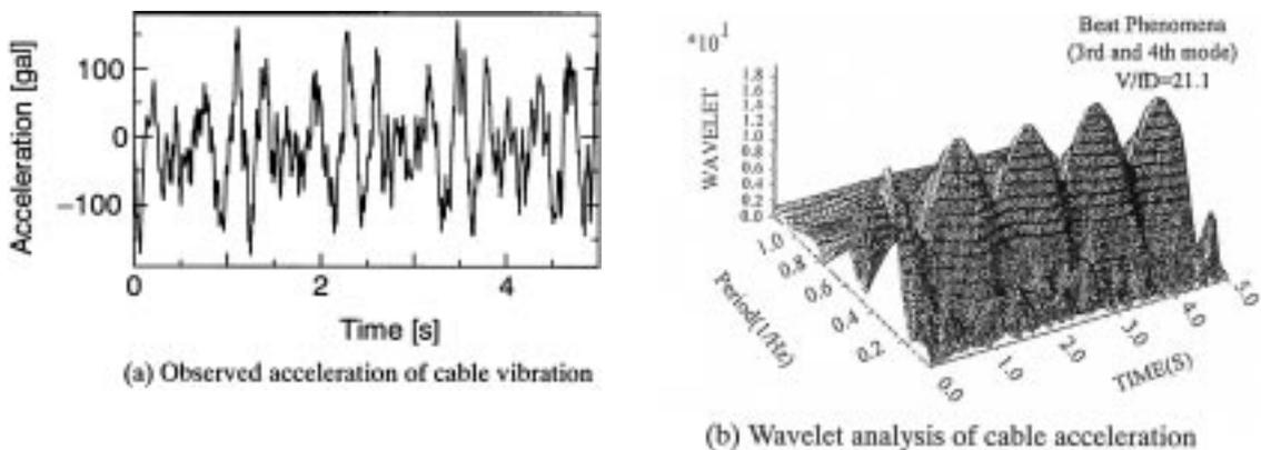
Fig. 4 Observed cable vibration at a prototype cable-stayed bridge
