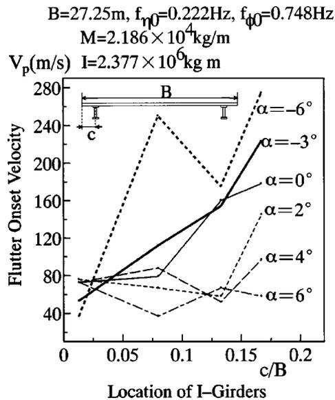
Fig. 6 Flutter instability depending on the location of edge girders and the angle of attack of wind
