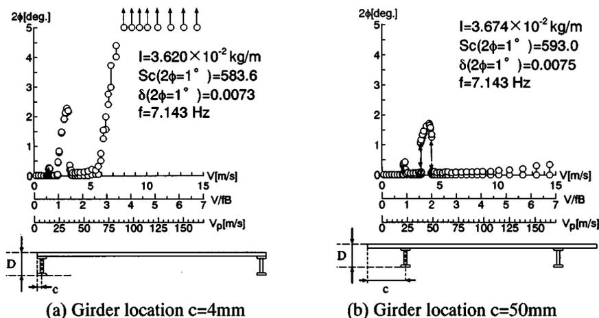
Fig. 7 Velocity - amplitude diagrams of the sections with two different girder locations (width  $B = 300$  mm, height  $D = 30$  mm, angle of attack  $\alpha = 0$  deg, torsional 1DOF, in smooth flow,  $V_p$ : field wind velocity on a certain long-span cable-stayed bridge with center span length of 610 m)
