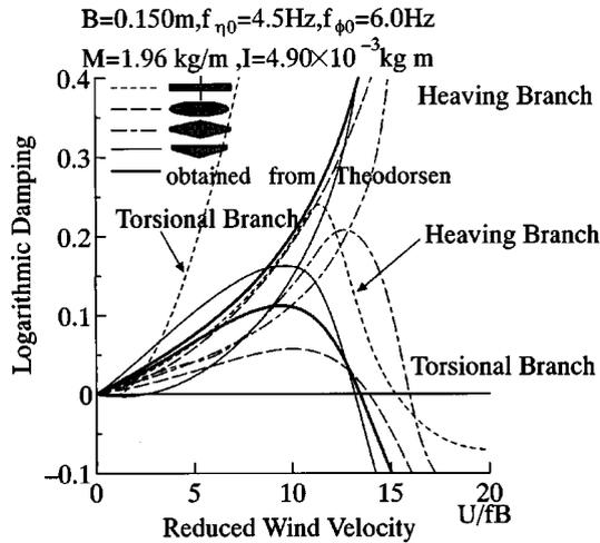
Fig. 10 Velocity - damping curve for the isolated deck sections
