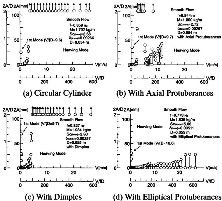
Fig. 3 Velocity - amplitude diagrams of cable models
