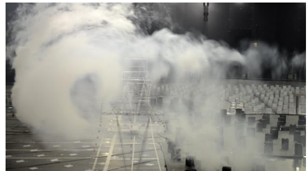
Fig. 4 Downburst formation snapshot at WindEEE
