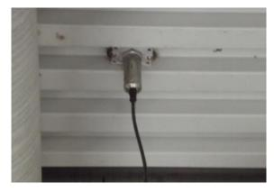
Fig. 4 wind-pressure transducer
