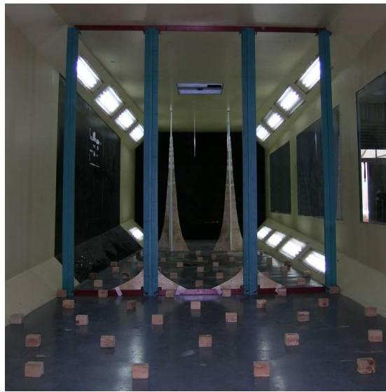
Fig. 4 Passive devices for simulating wind field of atmospheric boundary layer
