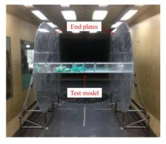
Fig. 1 Wind tunnel test model
