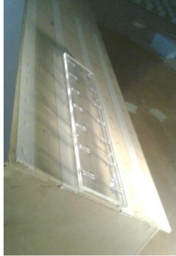
Fig. 5 Close-up view of the 22.5° roof pitch house model with a 1×7 solar panel array located at Position D in wind tunnel
