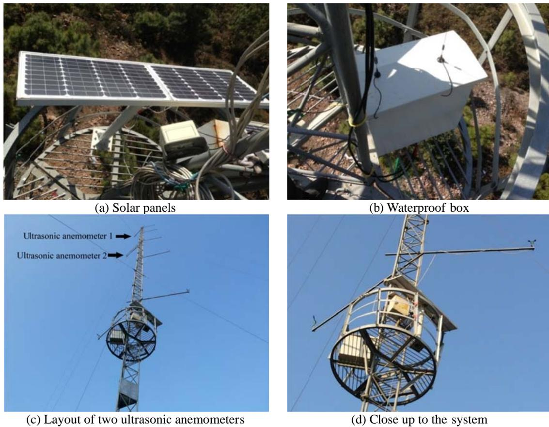
Fig. 6 Photos of field installation of proposed system
