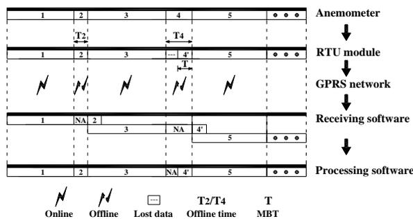
Fig. 2 Schematic diagram of data transmission and treatment
