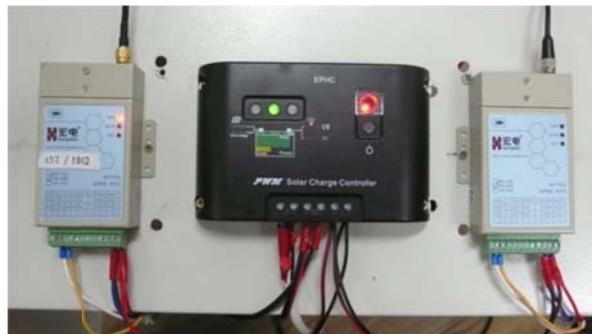
Fig. 4 RTU modules used in the field
