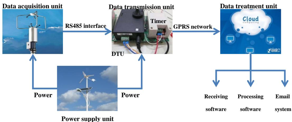
Fig. 1 Architecture of instrumentation system
