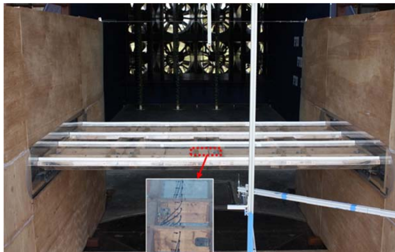
Fig. 4 1:36 scale model in front of Wall of Wind, Florida International University
