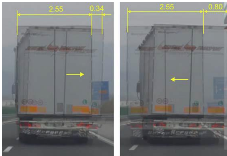
Fig. 5 Vehicle path deviations (m) for vehicle run 3 (Batista 2011)
