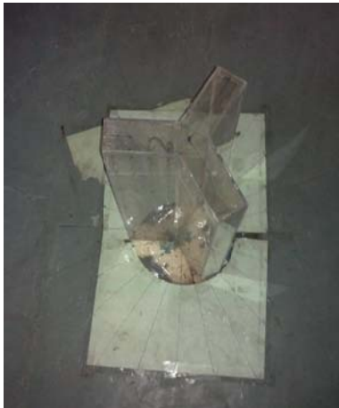
Fig. 2 Y- shaped models in boundary layer wind tunnel
