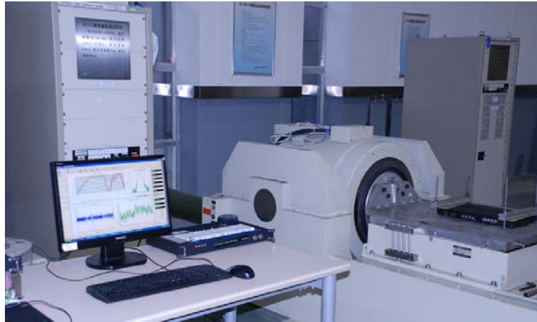
(c) Actual non-Gaussian vibration testing on the shaker
