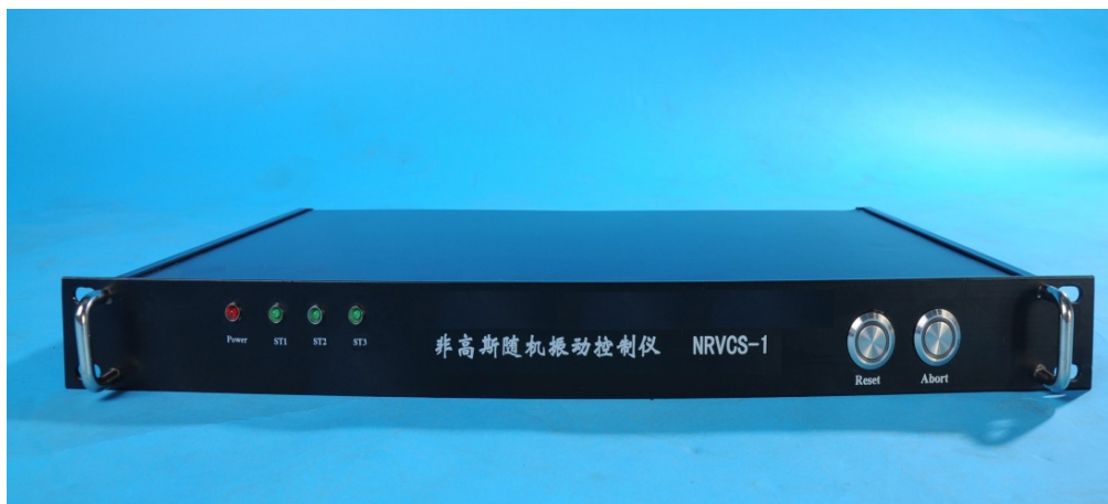
(a) Hardware of Non-Gaussian random vibration controller
