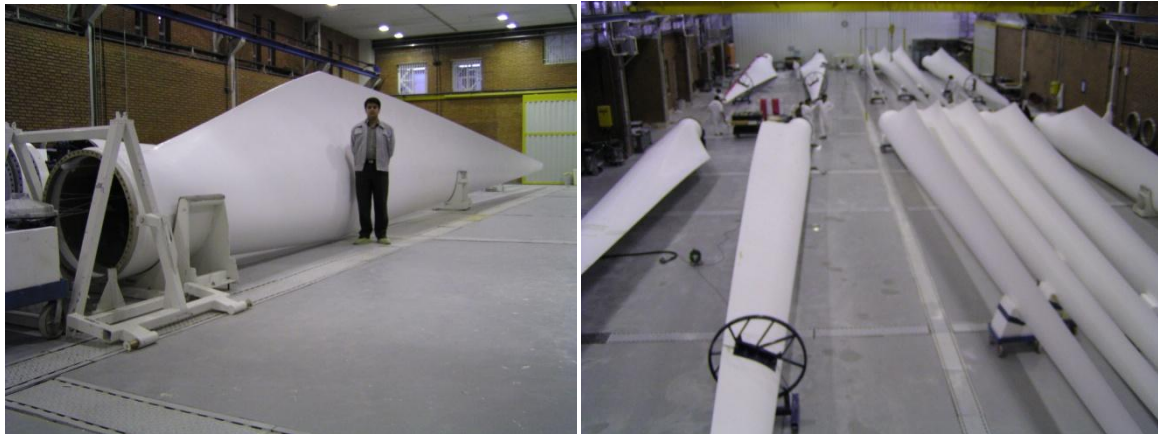
Fig. 1 23 meter blades belonging to 660 kW wind turbine (Courtesy of Sabaniroo Co., Iran)
