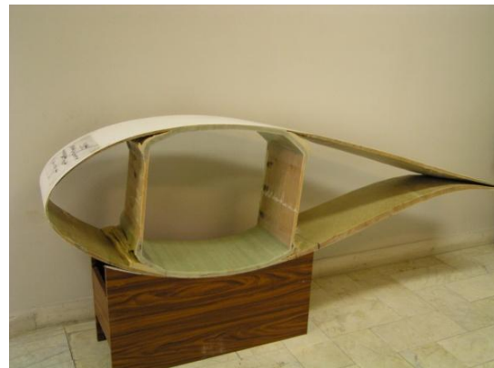
(b) Cut section of blade including shell and spar
