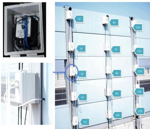
Fig. 4 Measuring points arrangements and instruments connection
