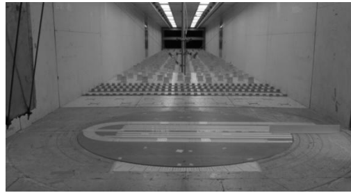
Fig. 7 Wind tunnel model of the noise mitigation structure at-grade (after Shum et al. 2011)
