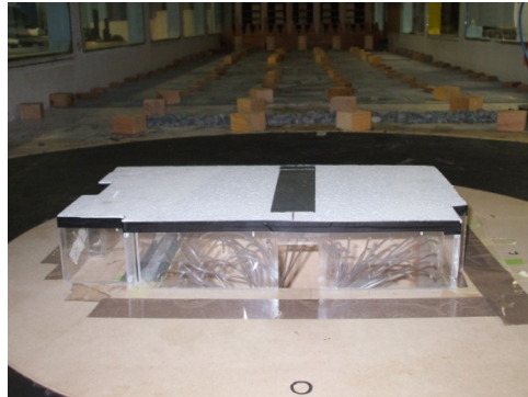
Fig. 6 Model with a flexible Styrofoam roof inside the de Bray wind tunnel
