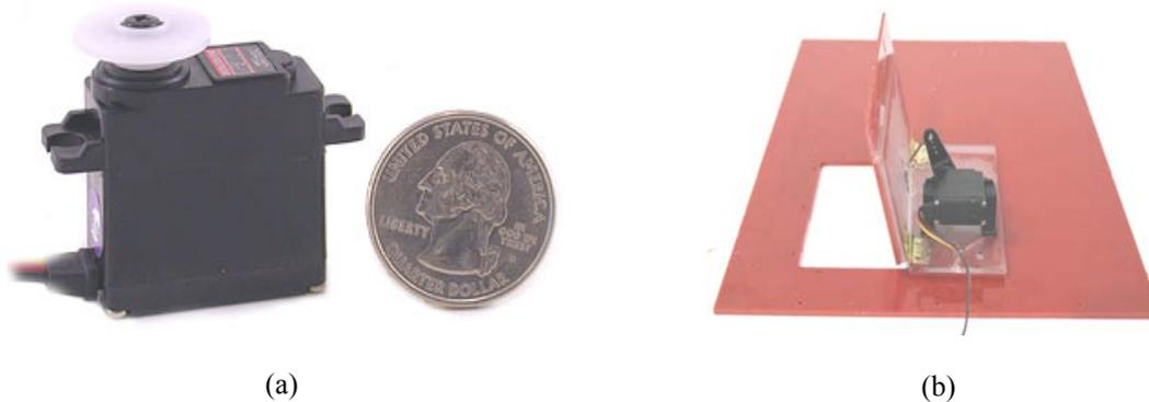
Fig. 4 Sudden failure simulation technique: (a) digital servo motor Hitec HSG-5084MG (courtesy of ServoCity™) and (b) window assembly and servo in open position
