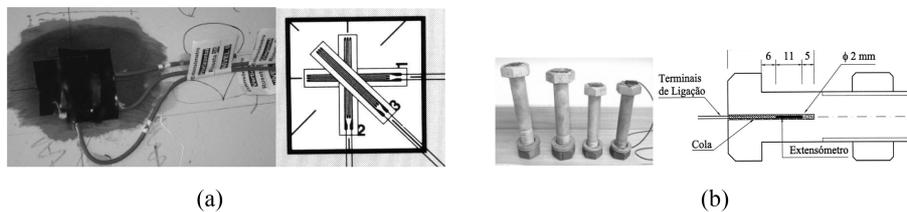
Fig. 2 Details of strain gauges : (a) Strain rosettes on the inner side of the shell and (b) strain gauges inside the bolts
