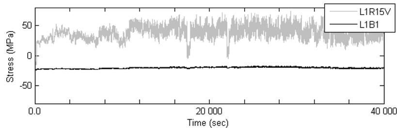
Fig. 7 Comparison between bolt stresses and shell vertical stresses at level 1
