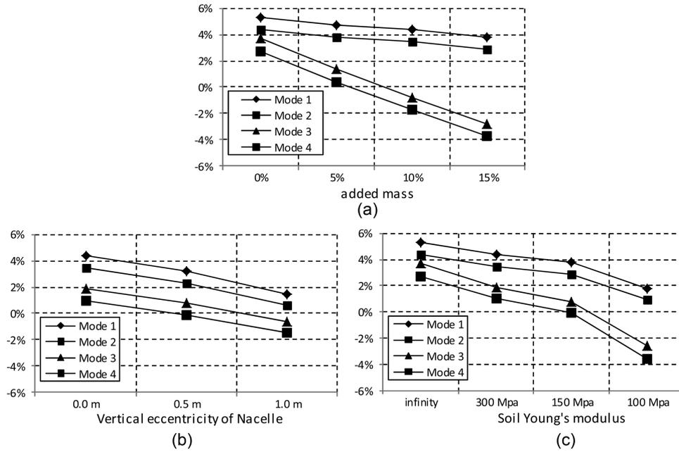
Fig. 9 Deviation of the natural frequencies in the FE model from measured results when varying: (a) mass, (b) soil stiffness and (c) vertical eccentricity of nacelle
