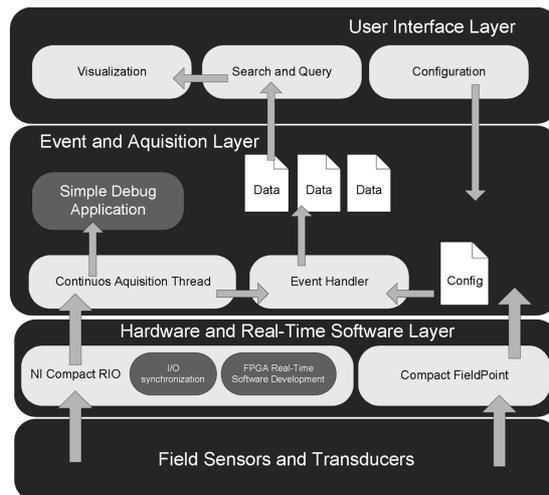
Fig. 4 Architecture of the LabView based computer application developed for synchronizing data loggers, signal decimation and recording
