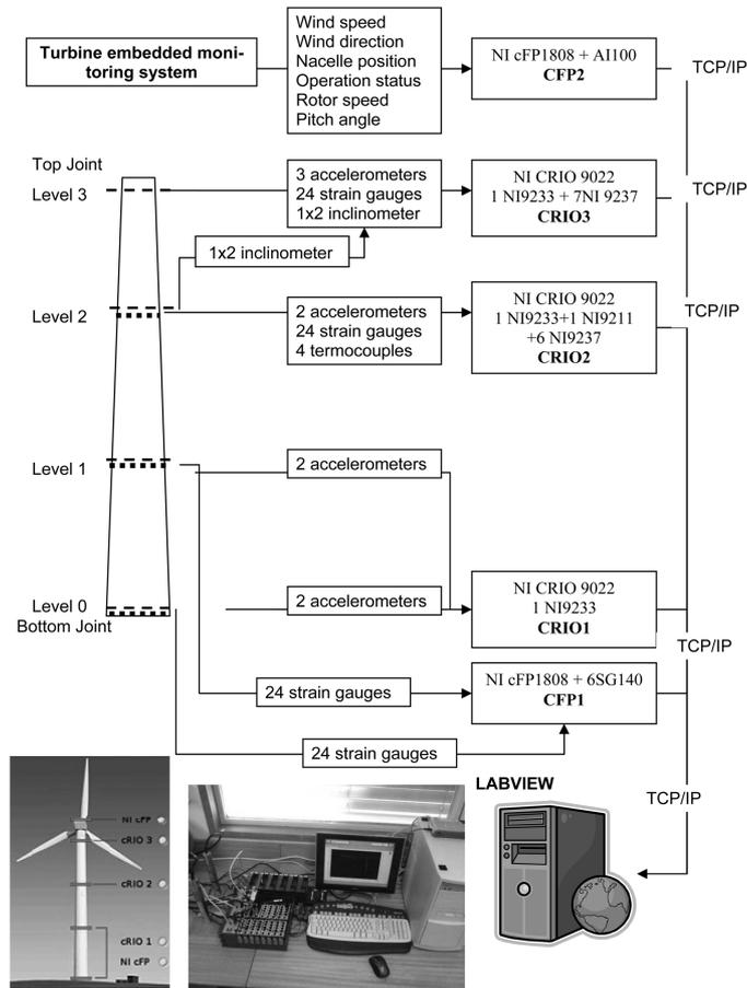
Fig. 3 Data logging and transmission inside the tower
