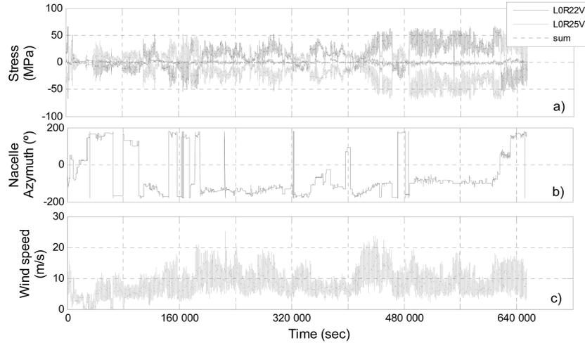
Fig. 6 Typical time histories: (a) vertical stress at points L0R22V and L0R25V and respective sum, (b) nacelle azimuth – positive clockwise from North direction and (c) wind speed at nacelle level
