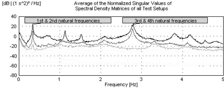
Fig. 8 Singular values of the spectral density matrices
