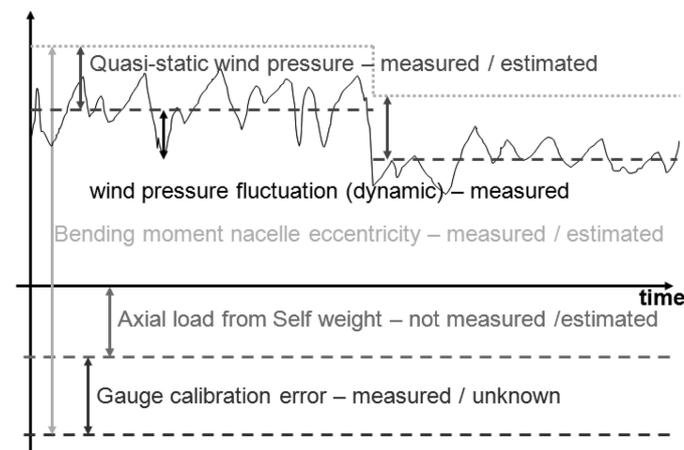
Fig. 5 Strain history at an arbitrary location and its decomposition in static or quasi-static components and dynamic component
