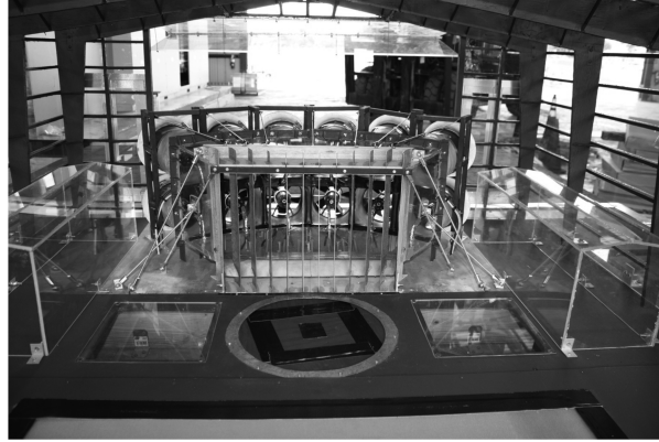
Fig. 1 Small-scale 12-fan Wall-of-Wind (WoW)
