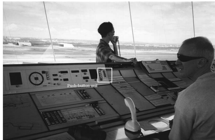
Fig. 2 Motion reporting push buttons in Brisbane Airport Control Tower
