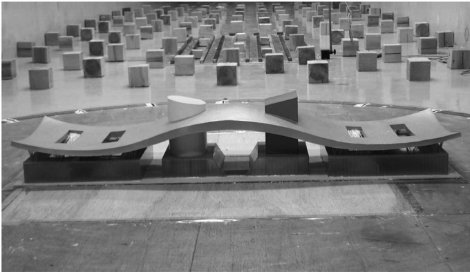
Fig. 3 The model of Shenzhen Citizen Center in the wind tunnel test
