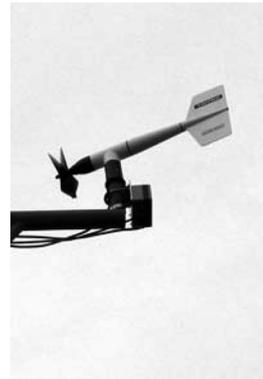
Fig. 2(b) Propeller anemometer
