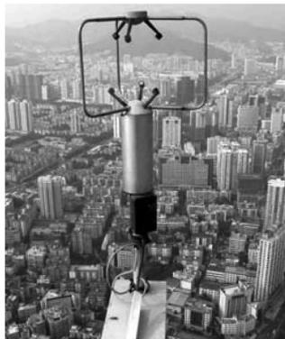
Fig. 2(c) Ultrasonic anemometer
