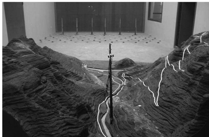
Fig. 13 1/500 scale model installed in the wind tunnel
