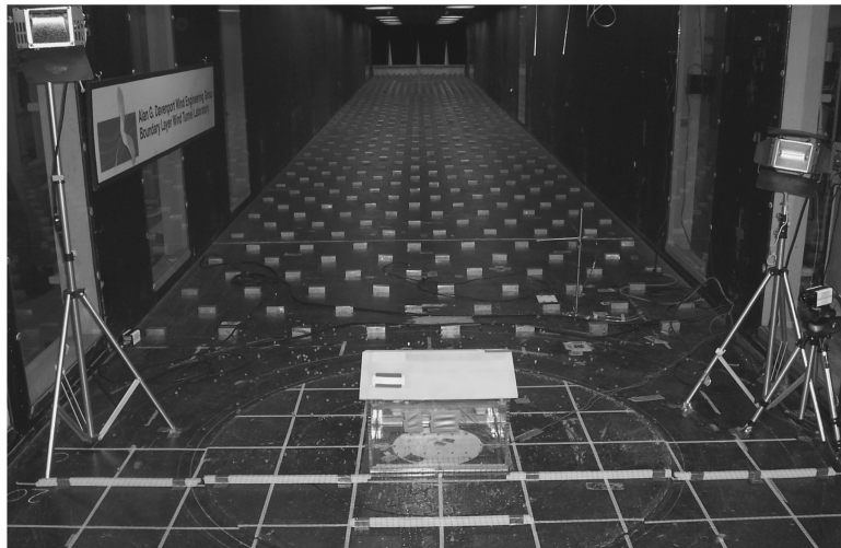
Fig. 2 Photograph of the model house in the wind tunnel, showing the upstream terrain simulation
