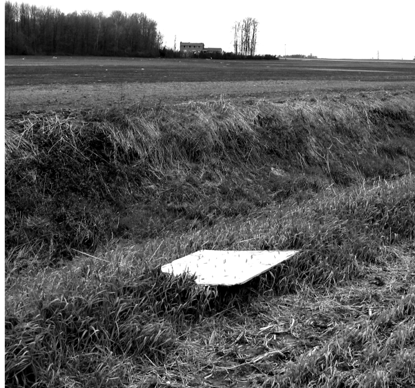
Fig. 1 Photograph of roof sheathing, caused by a downburst in Bornham, Ontario. The source of the plywood sheathing is the house shown in the background. This particular panel travelled about 450 m
