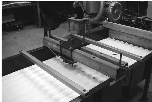
Fig. 9 Air box with double 900 mm span cladding installed
