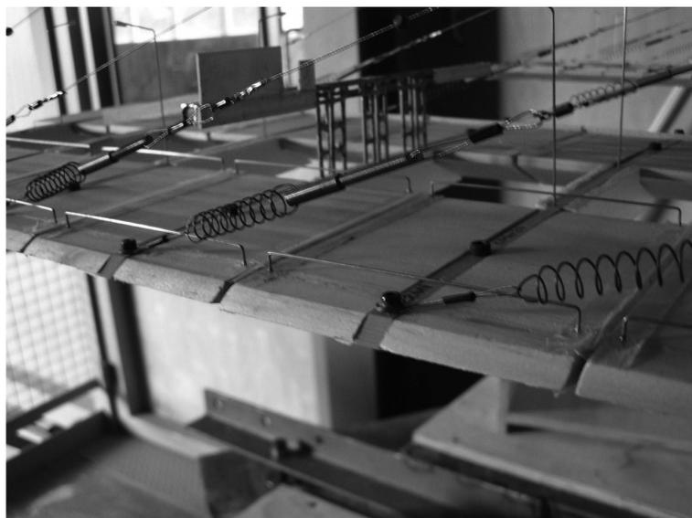
Fig. 7 Photograph of the deck in aeroelastic full bridge model with steel braces simulating railings
