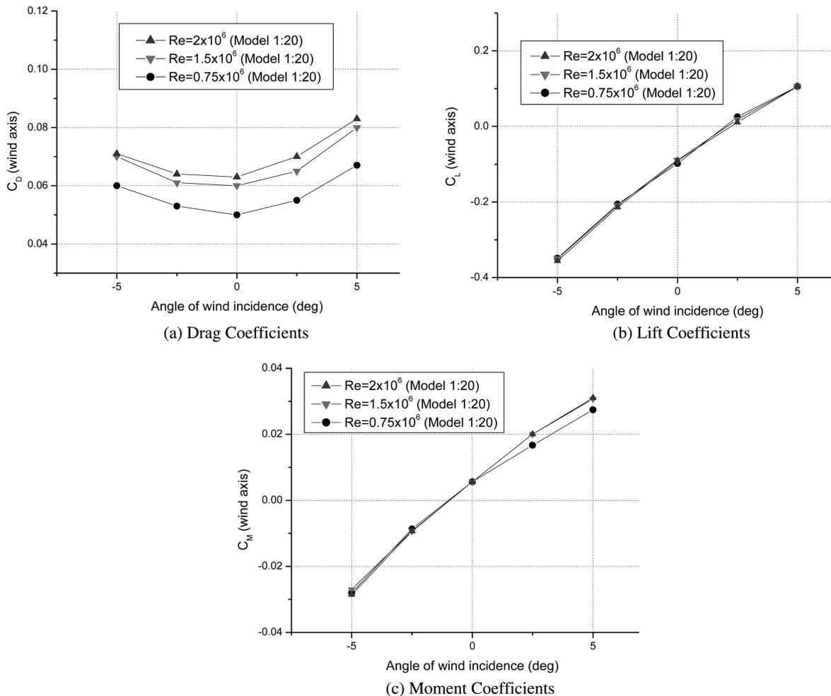
Fig. 6 Steady state wind load coefficients measured for the AJ cross section (1:20 scale) in smooth flow
