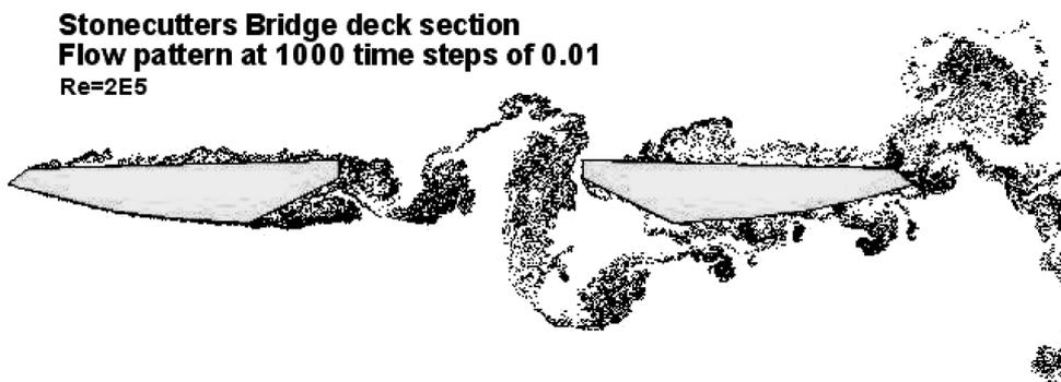
Fig. 11 Flow pattern at 1000 time steps of 0.01 for Stonecutters Bridge deck
