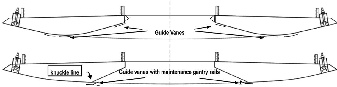
Fig. 2 Reference scheme (Top R-section) and final alternative (Bottom AJ-section) and guide vane configurations investigated
