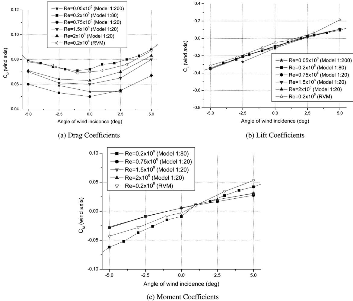
Fig. 12 Steady state wind load coefficients measured in wind tunnel experiments and calculated by RVM
