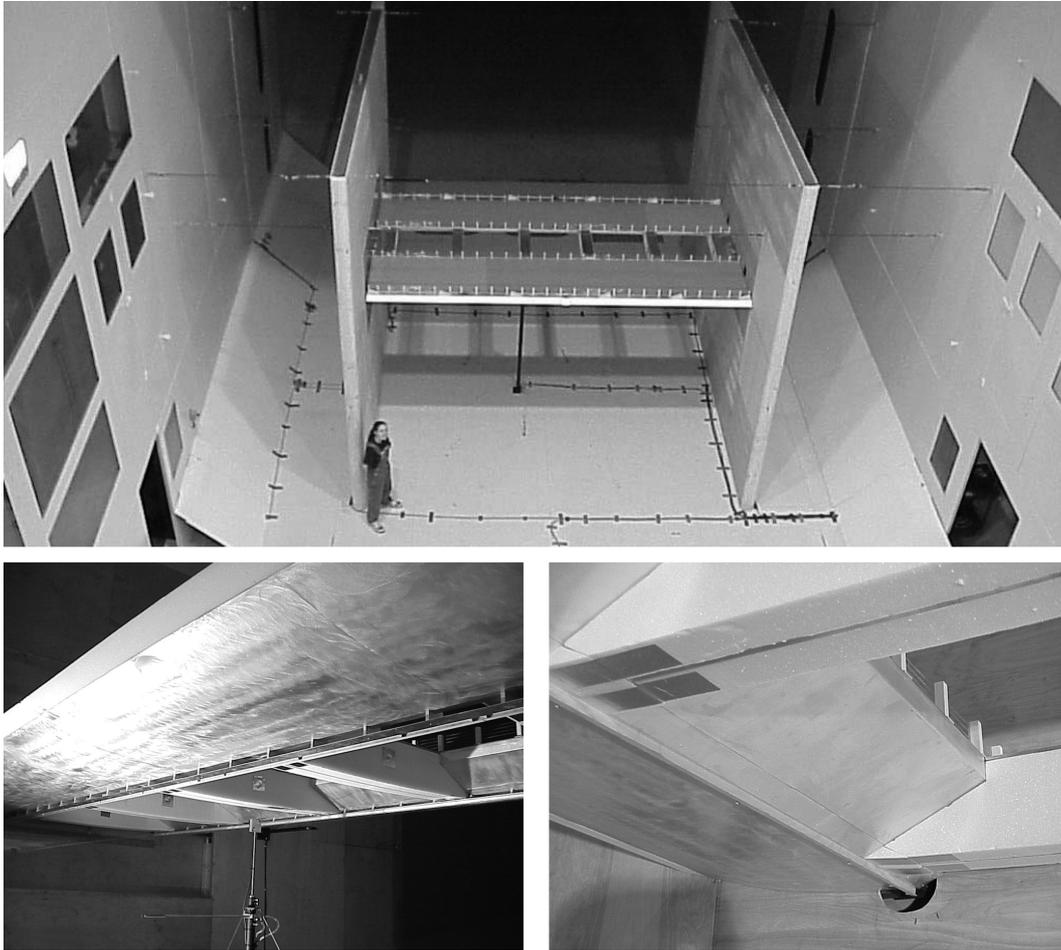
Fig. 5 1:20 AJ section model suspended in the NRCC  $9 \times 9$  m low speed wind tunnel (top). Details of guide vanes option 4 (bottom, left) and maintenance gantry rails (bottom, right).
