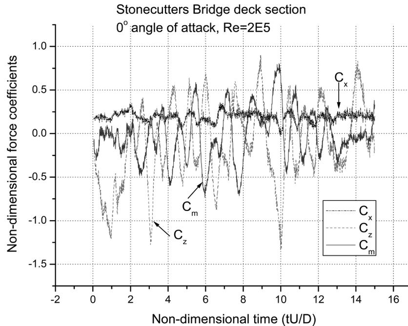
Fig. 10 Time traces of the development of  $C_x$ ,  $C_z$  and  $C_m$  for Stonecutters Bridge deck section
