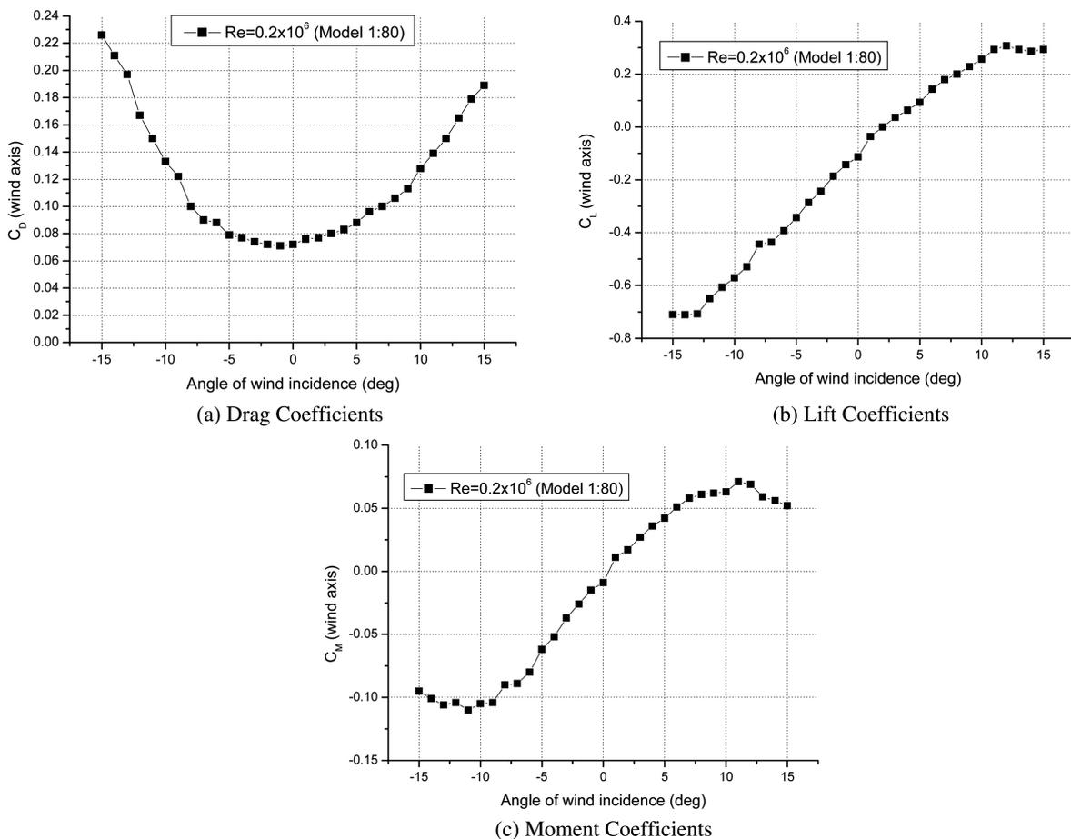
Fig. 4 Steady state wind load coefficients measured for the AJ cross section (1:80 scale) in smooth flow
