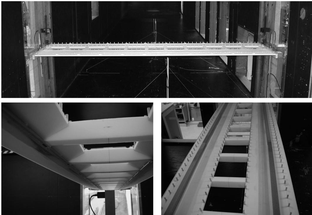
Fig. 3 AJ section model in the DMI  $2.6 \times 1.8$  m boundary layer wind tunnel (top). Details of guide vanes (bottom, left) and AJ with traffic models on the roadway (bottom, right)
