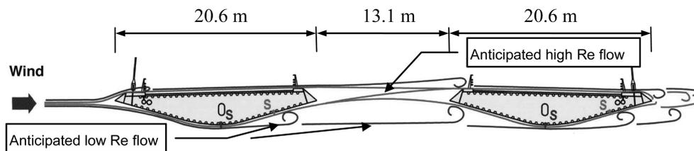
Fig. 1 Conceptual flow about the Stonecutters Bridge deck at high and low Reynolds numbers
